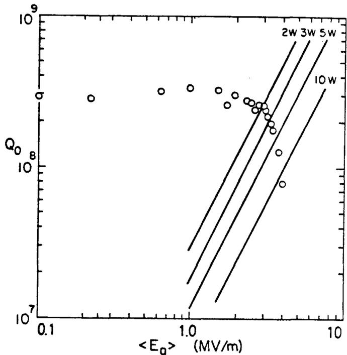
Fig. 2  $Q$  vs. Average Accelerating Field for tests of the low beta quarter wave resonator.
