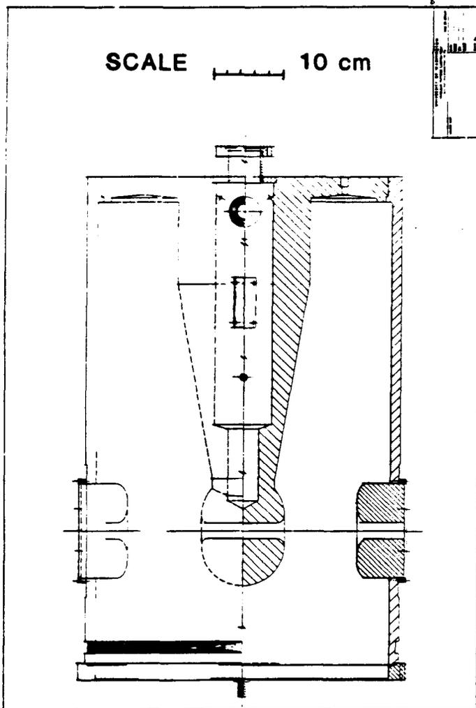
Fig. 3 The high beta quarter wave resonator.
