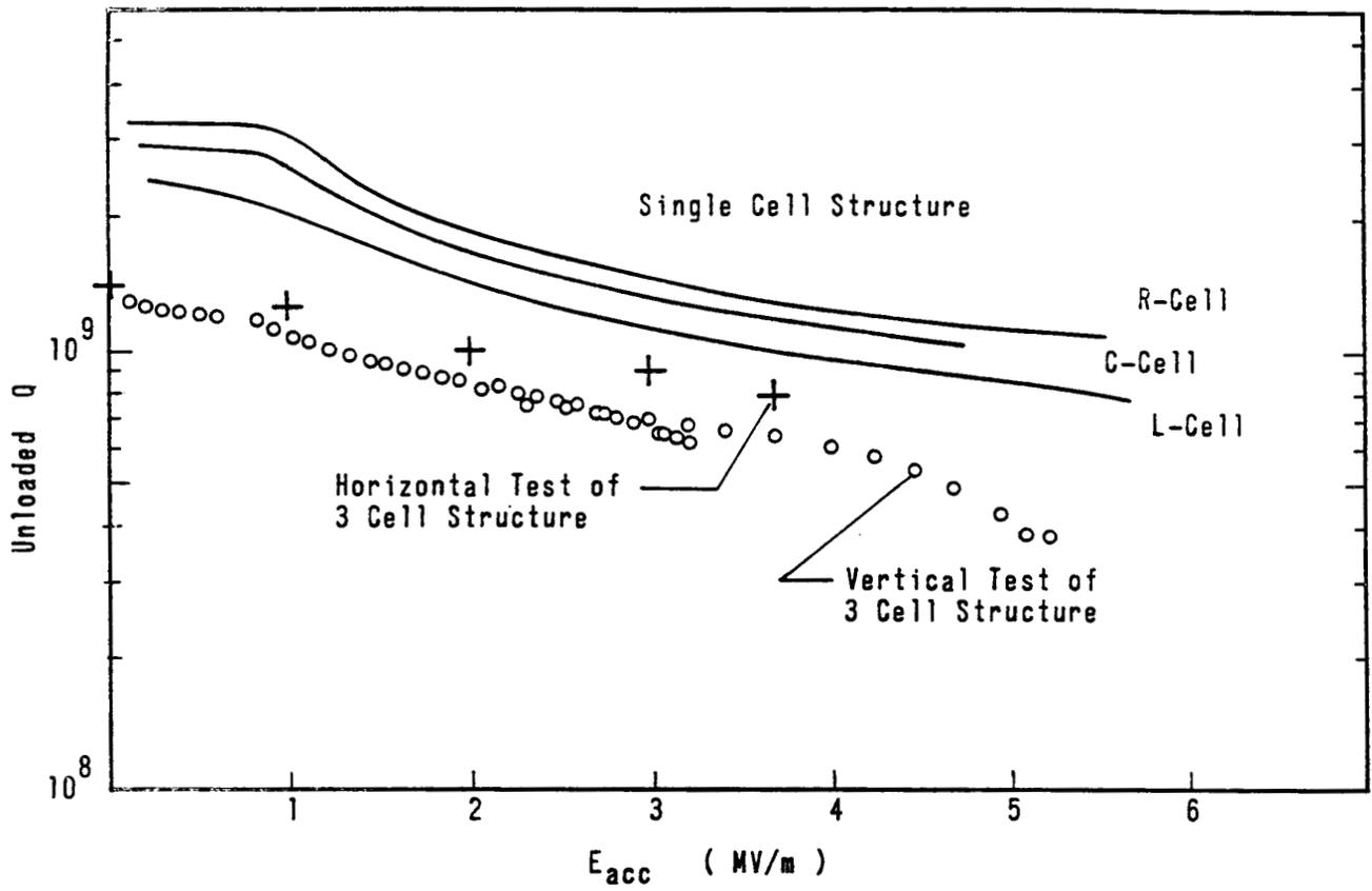
Fig. 4  $Q_0$  and  $E_{acc}$  of the three-cell structure.
