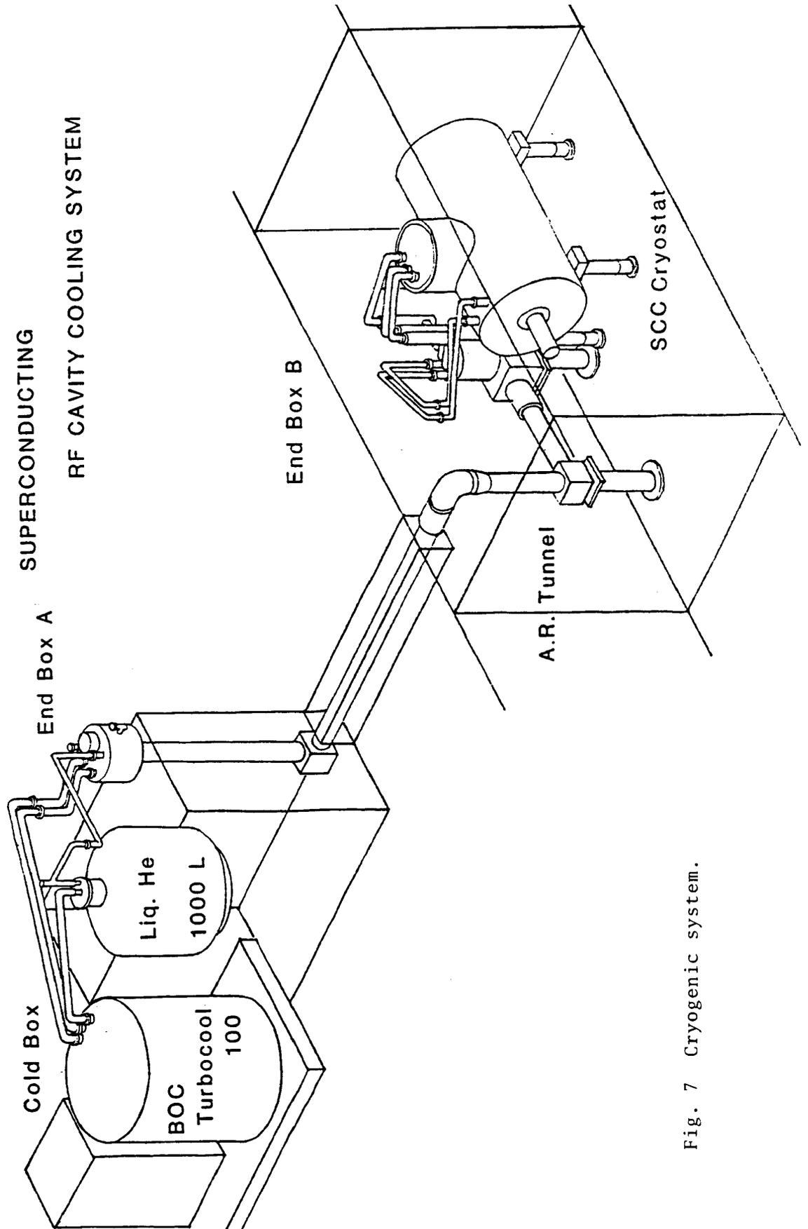
Fig. 7 Cryogenic system.
