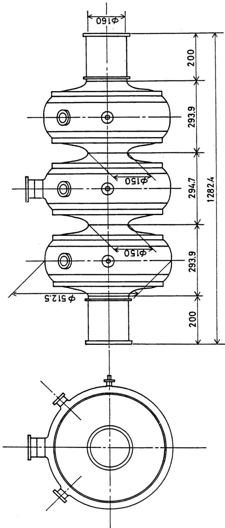
Fig. 3 A three-cell structure.
