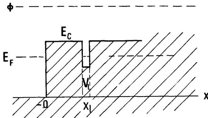
Fig. 5: Potential simulating a dielectric coating ( $E_c$  = lower edge of conduction band) on a metal, housing a localized state at  $x_{\ell}$ .  $\phi$  is the electron affinity of the metal having  $E_F$  as Fermi energy.
