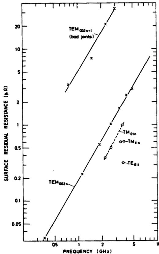
Fig. 8: Surface residual resistances  $R_{res}$  of lead plated Cu cavities:<sup>7</sup>
