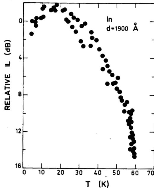
Fig. 6: Experimental <sup>30</sup> temperature dependence of the squared conversion efficiency  $\alpha^2$  (in dB) relative to its value at 4.2K for an indium film.
