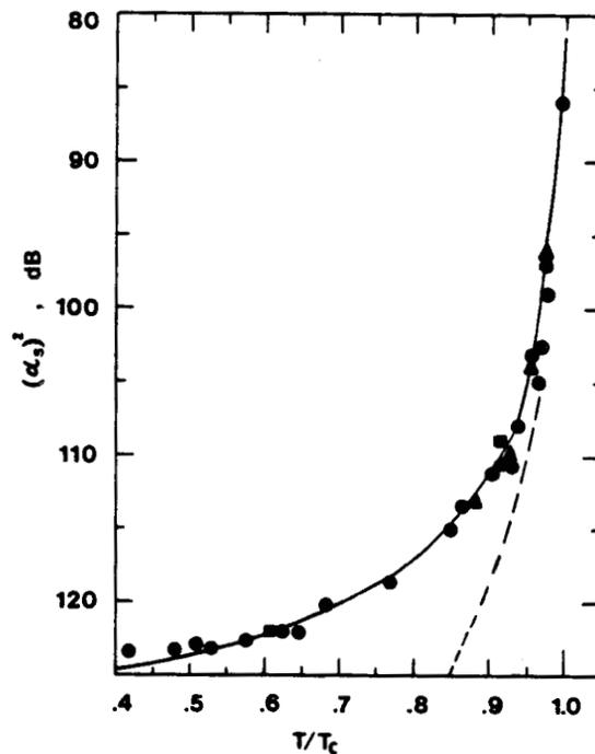
Fig. 7: Measured conversion efficiency squared  $\alpha_S^2$  versus reduced temperature  $T/T_C$  for a superconducting In film ( $T_C=3.4$  K). The theoretical curve (—) describes <sup>29</sup> the experimental data well assuming diffuse surface scattering for the whole wave function. The dashed curve (---) assumes diffuse surface scattering for the normal component  $n(T)/n_C \cong (1-(T/T_C)^4)$  only and cannot describe the experimental results.
