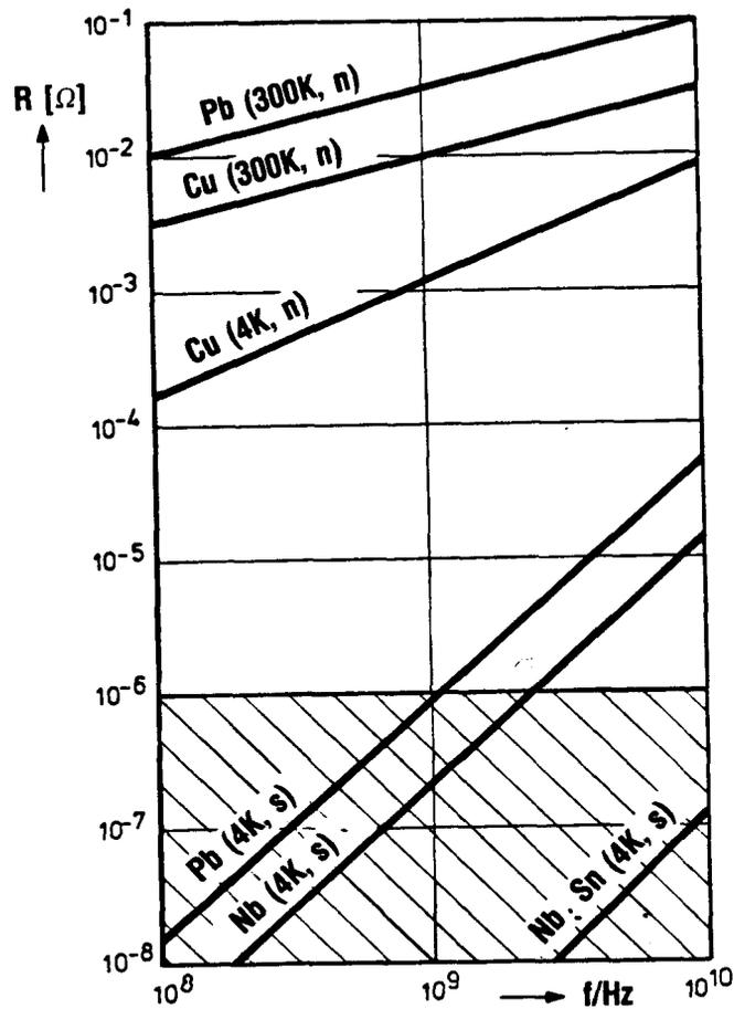
Fig. 1: Surface resistance of pure Pb, Cu, Nb and Nb<sub>3</sub>Sn at 300 K and 4 K in the GHz range. The strong reduction of R compared to R(Cu, 4K) is due to the energy gap  $2\Delta > 10^{11}$  Hz·h opening in the superconducting state. The shaded region indicates the appearance of additional - residual - losses  $R_{res}$ , e.g., due to dust, joints or interface states.
