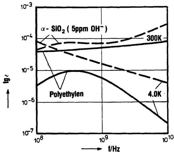
Fig. 4: Dielectric losses of amorphous dielectrics in the GHz range as described by the loss tangent  $\text{tg} \delta_E = \epsilon''/\epsilon'$
