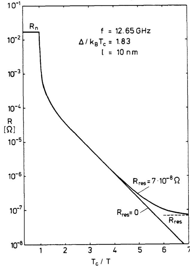
Fig. 2: The temperature dependence of the surface resistance of Nb at 12 GHz. The decrease of  $R(T)$  at  $T_c = 9.25$  K is stronger than exponential because the penetration depth  $\lambda_B(T \leq T_c)$  decreases rapidly also with lowering the temperature. Below about 4 K  $\lambda_B(T) \cong \text{const}$  holds and thus  $R_{\text{BCS}}(T) \propto \exp(-\Delta/kT)/kT$  describes the decrease of  $R(T)$  till the residual rf losses dominate below 2 K.
