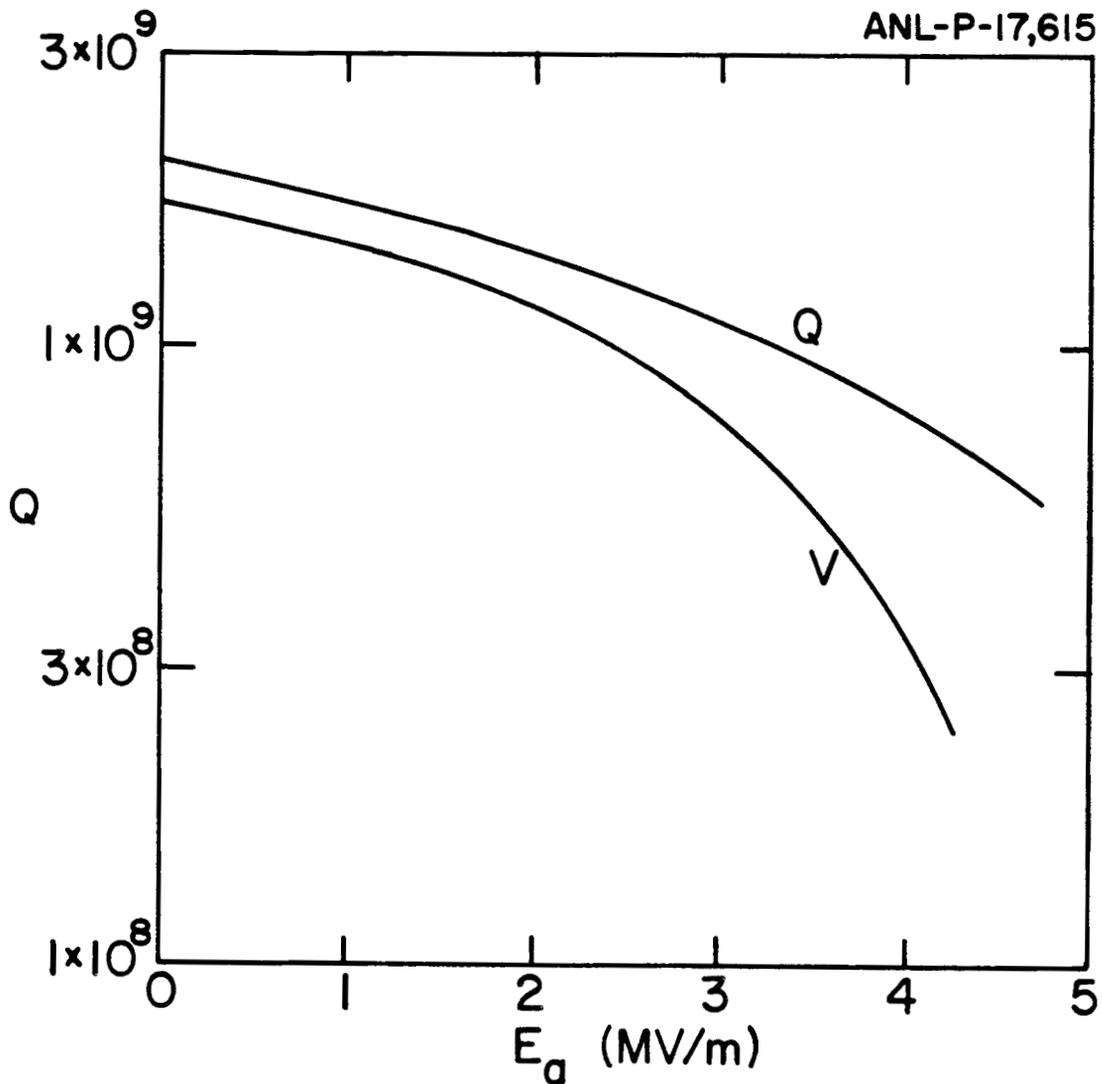
Figure 4. Resonator  $Q$  vs. accelerating field level  $E_a$ , measured at 4.2K. Curve V is for the V-type split ring resonator with an interior length of 35.6 cm. Curve Q is for a coaxial quarter wave line resonator with a 20.3 cm interior length.
