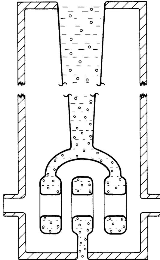
Figure 6. Cross-section of a conceptual design for a very low velocity superconducting resonator. The two high-voltage drift tubes are driven by a tapered coaxial line.
