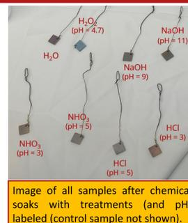
The niobium oxide structure plays a crucial role in the **binding of SnCl<sub>2</sub> to niobium during nucleation.** DFT calculations suggest that acidic solutions which remove OH groups will generate more SnCl<sub>2</sub> binding sites, **encouraging more uniform nucleation.**
