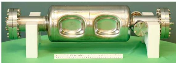
Figure 11: Final welded 2-cell rf-dipole cavity.
