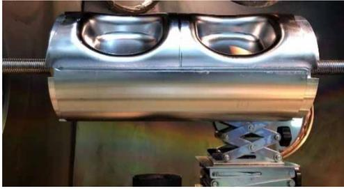
Figure 9: Center body welding in the EBW machine.
