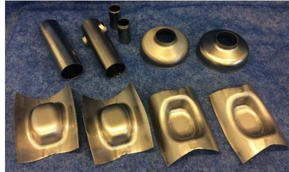
Figure 6: Formed poles, end caps and beam tubes.
