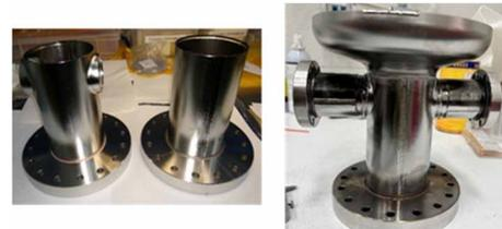
Figure 7: Beam pipes assemblies.
