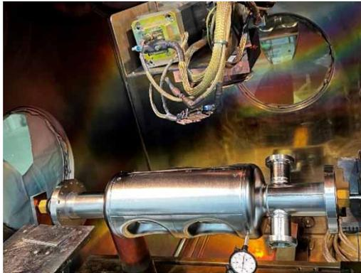
Figure 10: Final welding of the 2-cell rf-dipole cavity.
