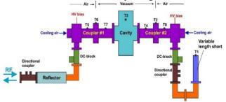
Figure 2: Schematic view of coupler test stand.
