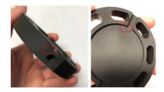
Figure 3: Flanges in Epoxy 82, fractures are visible near corners and sharp edges.
