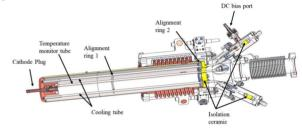
Figure 1: Cathode Stalk assembly [7].
