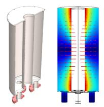
Figure 2: Model (left) and field distribution in the fundamental 389 MHz mode (right) for the HWR in Ref. [1].
