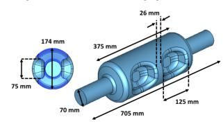
Figure 2: 952.6 MHz 2-cell rf-dipole cavity.
