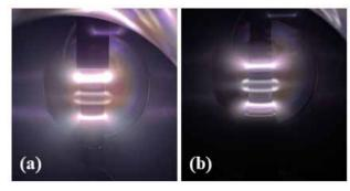
Figure 1: Photograph of stable plasma discharge at 10 mTorr using DC power (a) 30 W for Nb, (b) 8 W for Sn.
