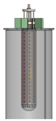
Figure 2: Conceptual setup of the coaxial Tmap system: 8 boards with each 19 sensors are arranged in a 45deg pattern to cover the inner conductor surface of the QWR. An actuation mechanism expands the system and presses the sensors against the cavity wall.
