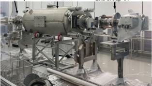
Figure 1: 56 MHz quarter-wave resonator cryomodule immediately before final clean assembly in the BNL class 10 clean room.
