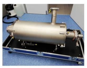
Figure 1: ESS high-beta 704 MHz cavity.
