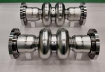
Figure 1: Fabricated niobium double-cell cavities.
