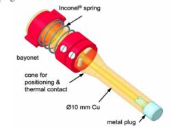
Figure 1: Cathode plug with plug tip, Cu body and bayonet structure.
