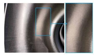
Figure 2: A part of the half-cell of an as-received HB650 cavity: Photograph captured with a digital camera inserted manually inside the cavity (left). Zoom-in image showing minor scratches (right).
