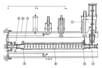
Figure 2: Sectional view of a cut in half cryomodule of the S-DALINAC . (1) Coaxial rf transmission line, (2) Coaxial input coupler, (3) Cavity tuning frame, (4) 20-cell elliptical cavity, (5) rf output coupler, (6) 80 K shielding, (7) 2 K helium vessel [3].
