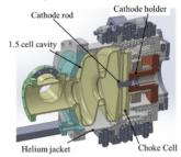
Figure 1: Structure of the KEK SRF gun #2.
