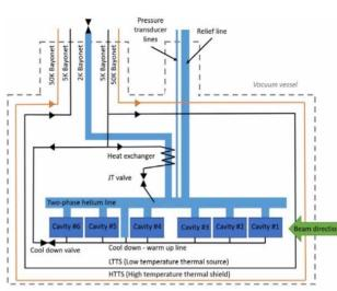
Figure 1: HB650 cryomodule layout.
