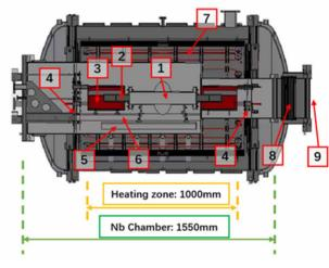
Figure 1: Overall design of the coating system at SARI:1 Nb cavity, **2** Sn crucible, **3** Crucible heater, **4** Nb reflectors inside Nb chamber, **5** Bracket rails, **6** Cavity bracket, **7** Mo heater of furnace, **8** bellows, **9** Pumping port for Nb chamber.
