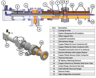
Figure 1: The full ppSSR2 coupler assembly.
