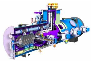
Figure 1: The LB650 cryomodule.
