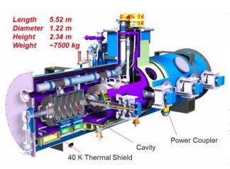
Figure 1: LB650 cryomodule layout.
