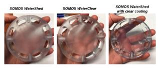
Figure 2: Comparison between clear flanges.
