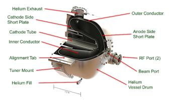
Figure 1: SRF Gun Cavity with key components.
