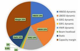
Figure 1: PIP-II linac total heat load includes the static, dynamic, beam, and static heat loads.
