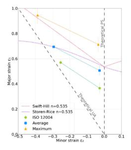
Figure 1: FLC for OFE-copper, 4 mm thick sheet [3].
