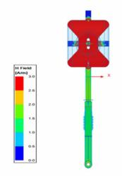
Figure 1: Magnetic field map@1 W for the coupler mounted in the SSR with  $\beta \sim 1$ .
