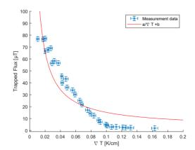
Figure 1: Measurement data of trapped flux versus temperature gradient during cooldown. The data is obtained using a large grain sample consisting only of two grains (sample dimension:  $(100 \times 60 \times 3) \text{ mm}^3$ ). Additionally, a fit according to the prediction in Ref. [2] is performed and the result is depicted in red.
