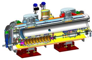
Figure 2: BCC cryomodule cross sectional view.
