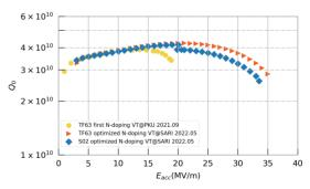
Figure 2: Vertical test results at 2 K of the two single-cell cavities, S02 and TF63.
