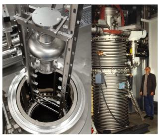
Figure 1: Single-cell Cavity inserted in the niobium-retort furnace (left side). External view of the niobium retort furnace during the initial assembly at DESY (right side).
