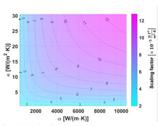
Figure 2: Scaling factor produced for a given combination  $\frac{\alpha}{2}$  of Kapitza conductivity and bulk thermal conductivity. Expected values include  $\alpha = 1000 - 3000 \text{ W} / (\text{m}^2 \cdot \text{K})$  and  $\frac{\alpha}{2} = 5 - 40 \text{ W} / (\text{m} \cdot \text{K})$  [3–5].
