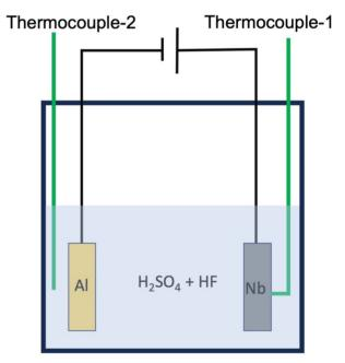
Figure 1: Schematic of the EP setup. Thermocouple-1 and -2 used to measure temperature of Nb sample and acid, respectively.
