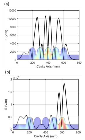
Figure 1: Electric field profile of two TE211 modes of interest on the axis of the C75 cavity, (a) 2656 MHz and (b) 2724 MHz.
