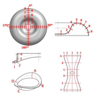
Figure 1: Points' location where the thickness is measured.
