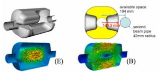
Figure 1: RFD cavity geometry (above left and right) and the electric and magnetic field patterns of its TE11-like deflecting mode (below left and below right).
