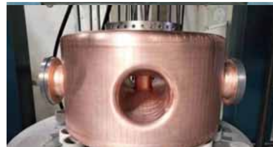
Spoke021 cavity coating with copper
