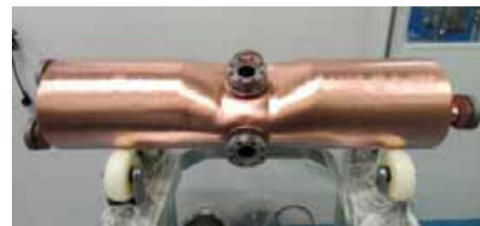
HWR010 cavity coating with copper
