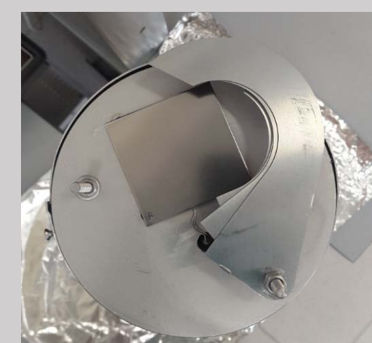
A sample and sputter assembly for the Nb deposition at INFN
