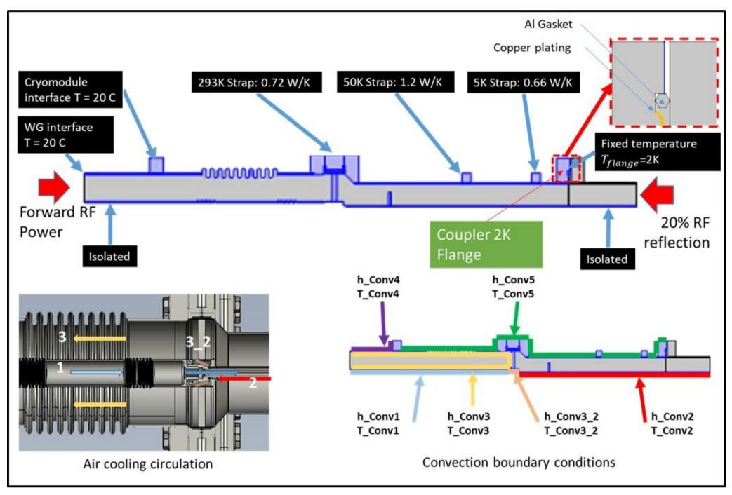
Power Coupler 2D axisymmetric model and boundary conditions
