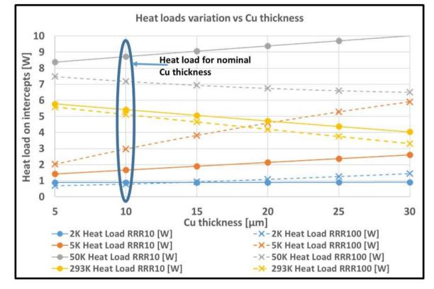
Heat loads vs Cu plating thickness and RRR
