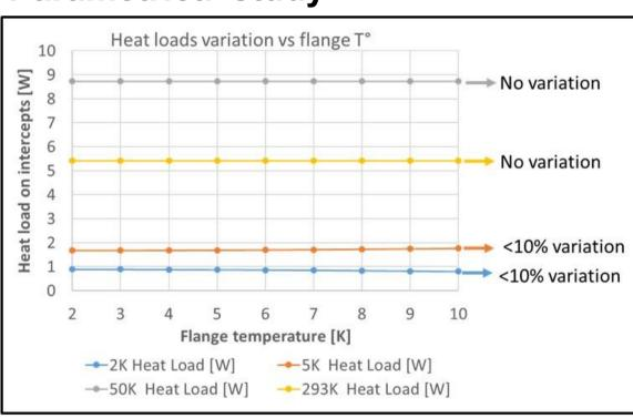
Heat loads vs the "2K flange" temperature
