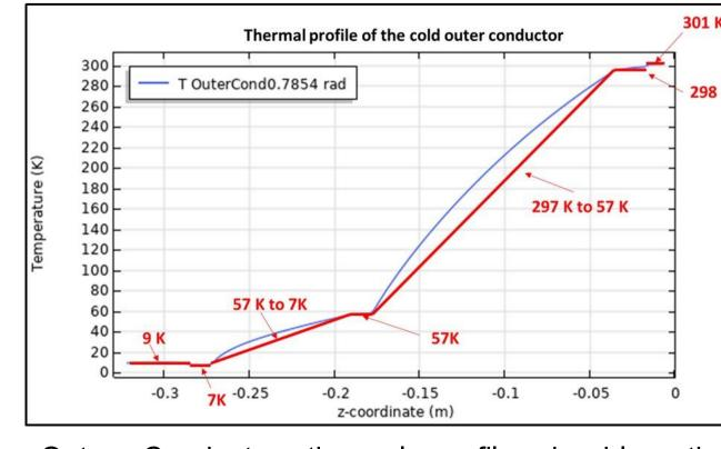
Outer Conductor thermal profile: in blue the calculated profile, in red the applied approximate profile
