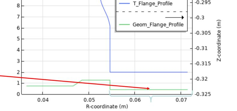
Although the boundary temperature set at 2K on one side of this flange, it was found that surfaces exposed to RF could reach more than 9 K for the phase generating the highest PC heat load towards the cavity. This temperature could reach 13 K if the set temperature is increased from 2K to 10 K. The temperature limitation to 13K could be explained by the contribution of the 5 K intercept.
