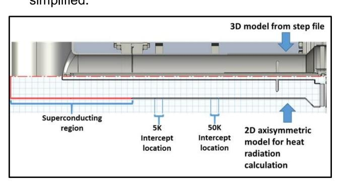
Thermal radiation calculation model
