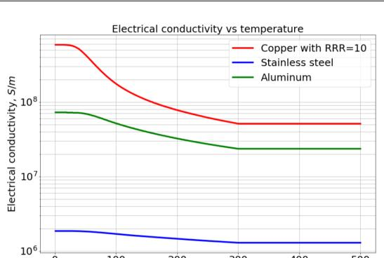
Electrical conductivity vs temperature
