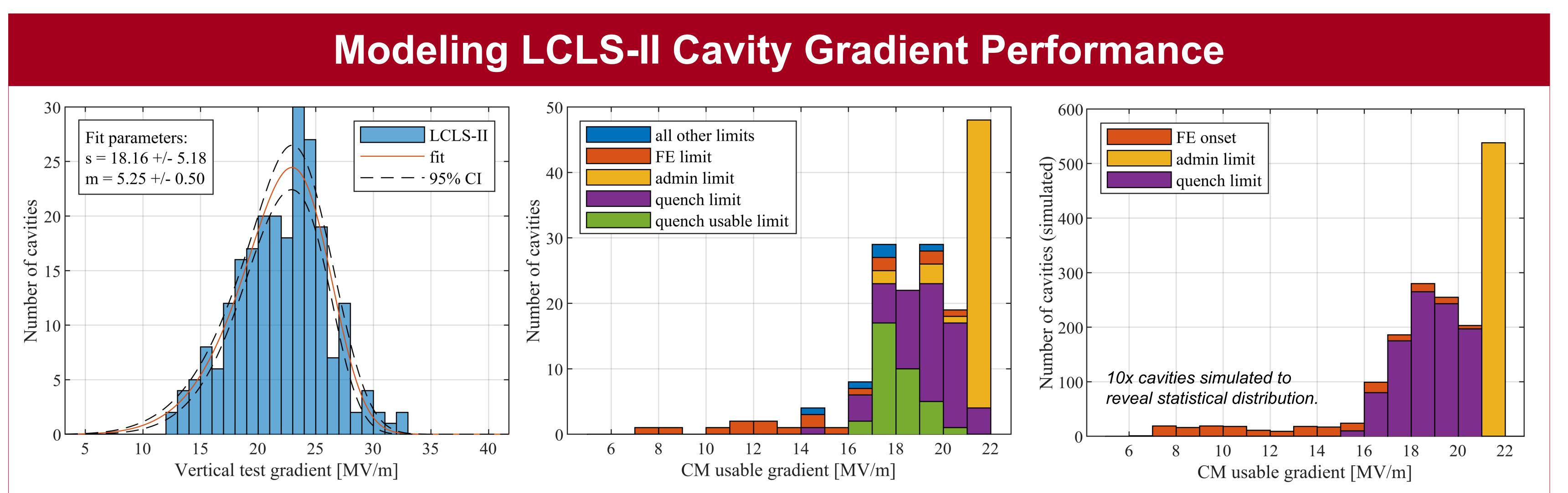
Peak vertical test accelerating gradients of LCLS-II cavities are well fitted by a two-parameter **thermal defect model**.
