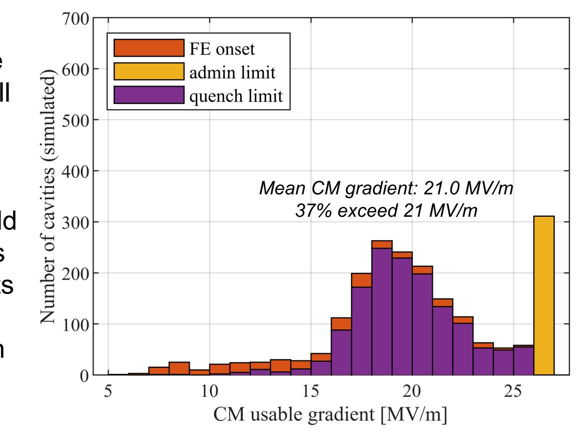
Simulation of LCLS-II-HE cryomodule gradients with improved vertical test gradients and rates of multipacting and field emission decreased by 50% The administrative limit on gradient has been increased to 26 MV/m, allowing the highperforming cavities to compensate for any low-gradient cavities.
