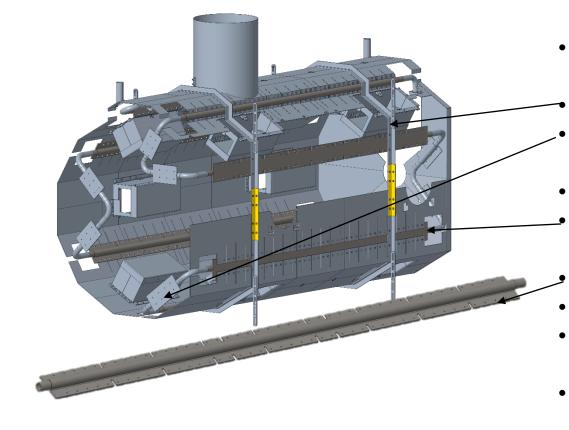
absorber support frame + inside piping for easy assembly bolted plates welding cooling Insulation
