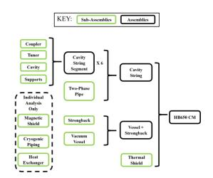
Figure 4: Analysis and combination scheme of components.
