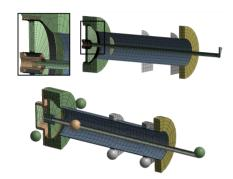
Figure 5: Section views of detailed (top) and simplified (bottom) coupler models.
