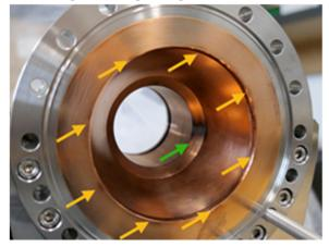
Figure 10: CsB upstream side and taper after operation.
