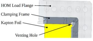
Figure 9: Detail of the diaphragm and its support frame. Venting holes in each corner also avoid creases in the foil.
