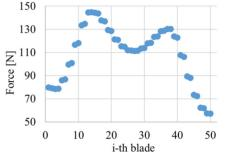
Figure 7: Force distribution on the 50 blades displayed for one tuner ring with 5 kN applied.
