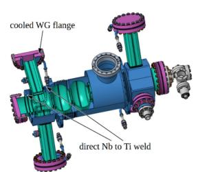
Figure 5: Cavity with ancillaries for cold test (Nb structure in green, NbTi flanges in pink and Ti parts in blue).
