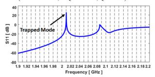
Figure 4: Reflection coefficient of the bellow for the TM mode excitation at the beampipe port.
