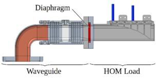
Figure 8: Waveguide with HOM load and diaphragm.
