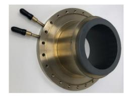
Figure 2: HOM absorber with cooling jacket (photo: courtesy of Xelera).
