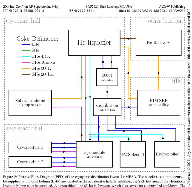
Figure 2: Process Flow Diagram (PFD) of the cryogenic distribution layout for MESA. The accelerator components to be supplied with liquid helium (LHe) are located in the accelerator hall. In addition, the SRF test area of the Helmholtz Institute Mainz must be supplied. A supercritical line (SHe) is foreseen, which also serves for a controlled cooldown. The gaseous phases (GHe) are color-coded according to their temperatures (light blue and orange) and pressures (magenta and brown).
