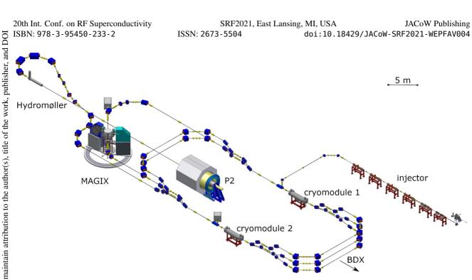
Figure 1: MESA lattice. Electrons are produced and pre-accelerated to 5 MeV in the injector before they are injected into the recirculating main-accelerator. The cryogenic components are the P2 experiment (solenoid and target), the hydromøller for polarization measurements, as well as the cryomodules. The BDX experiment is positioned outside of the accelerator hall, but in line with the P2 beam dump and not shown in this picture.
