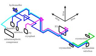
Figure 3: Piping path for connecting the cyoplant hall above ground with the accelerator hall below ground. The old building structure is limiting the possible paths [9]. Dark blue represents the liquefier connection to the cryomodules valve box and P2 solenoid, green the distribution from the cryomodule valve box to the modules, light blue the 16 mbar string and magenta the P2 target cooling circuit.
