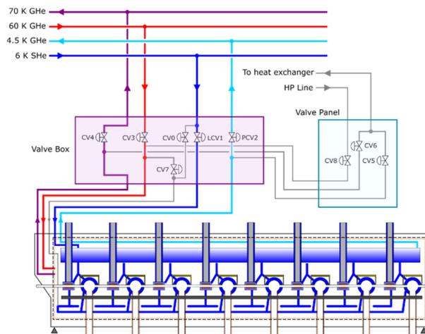
Figure 7: Principle of the cryogenic circuits of the IFMIF-DONES cryomodules with the flow of fluids in nominal operation. Note that LCV1 is the Joule-Thomson valve and that the valves needed for the cool-down process are also represented.
