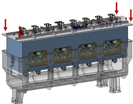
Figure 6: Insertion of the cold mass inside the vacuum vessel for the IFMIF-DONES cryomodules.
