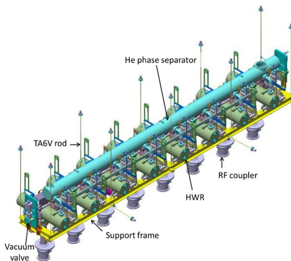
Figure 3: Cold mass of the IFMIF/EVEDA cryomodule.
