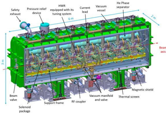
Figure 2: Overview of the IFMIF/EVEDA cryomodule.
