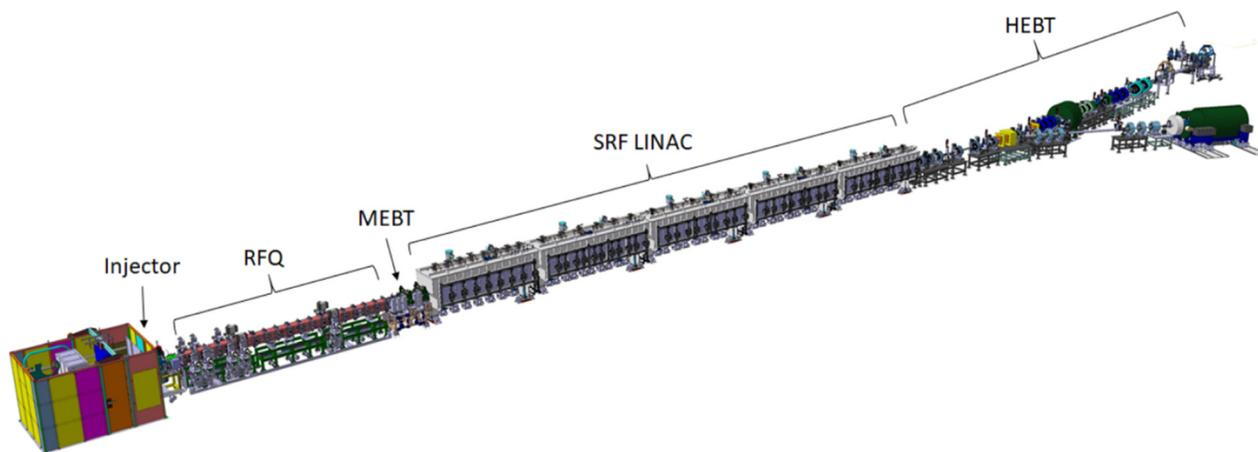
Figure 1: Layout of the IFMIF-DONES accelerator.
