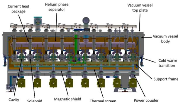
Figure 5: Overview of the IFMIF-DONES cryomodules (example of the first low-beta cryomodule CM1, the design principle is similar for the others).
