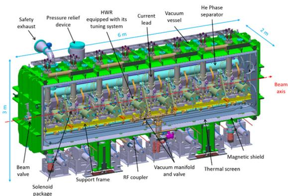
Figure 2: Overview of the IFMIF/EVEDA cryomodule.
