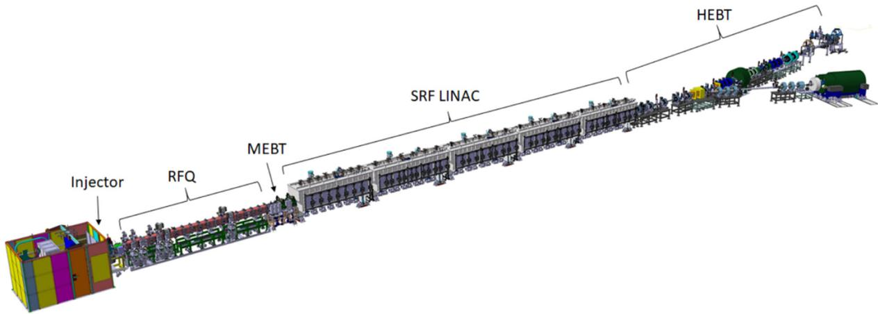
Figure 1: Layout of the IFMIF-DONES accelerator.
