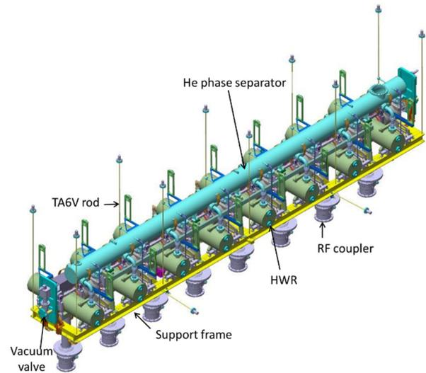
Figure 3: Cold mass of the IFMIF/EVEDA cryomodule.
