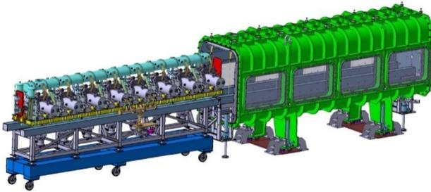
Figure 4: The two main sub-assemblies before the insertion of the cold mass inside the vacuum vessel.
