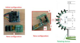
Figure 4: Set of three sensors, initial and old configuration (left), rotating frame with 9 sets (right).
