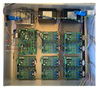
Figure 5: Electronic card for the 27 sensors.
