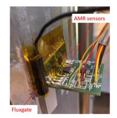
Figure 1: Set of three AMR sensors (X, Y and Z) and fluxgate installed on a cavity.
