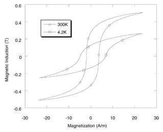
Figure 3: Mumetal torus magnetization as a function of applied field at two different temperatures [6].
