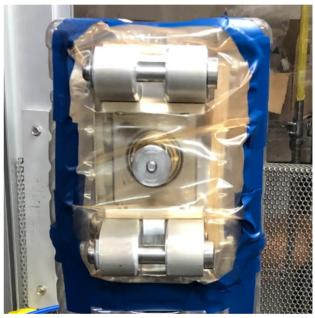
Figure 7: Opener Stirrups, Piston & Membrane.
