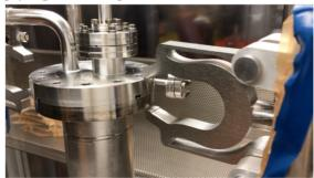
Figure 4: Clamp Openers applying Model 1 Clamps.
