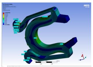
Figure 5: Model 1 Clamp's ANSYS Stress Results.
