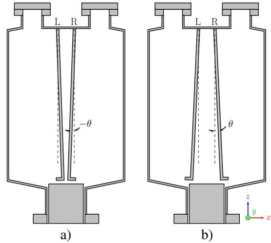
Figure 3: Schematic diagram of the angle variation of the Nb rods. The rotation of the rods was done around the  $y$ -axis with an angle  $\theta$  that is a) negative when the rods get closer and b) positive when the rods draw apart.
