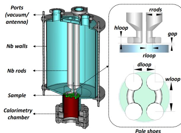
Figure 1: Cross-sectional view of a QPR (left) with the parametrized model of the pole shoes (right) [14].
