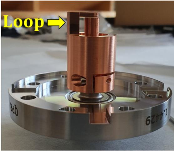
Figure 8: Input antenna: the coupling is controlled via the angle between the loop area and the field orientation.
