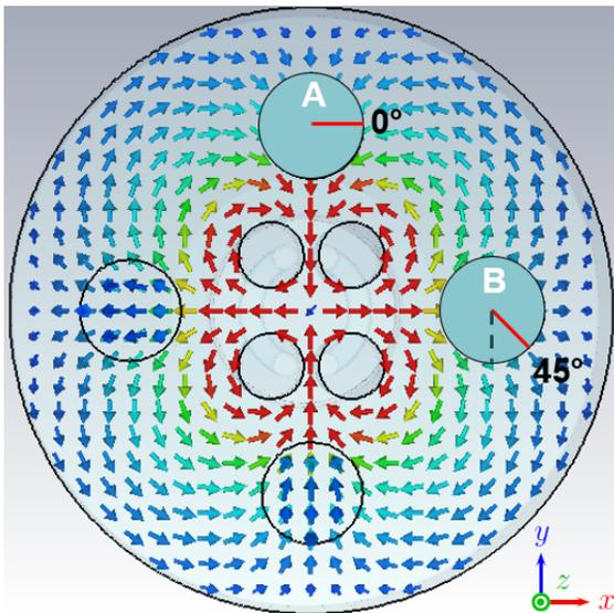
Figure 9: Cutting plane of the QPR normal to the  $z$ -axis. The input antenna loop area was fixed at  $0^\circ$  in port position A and the probe oriented at  $45^\circ$  in B. The magnetic field distribution corresponds to a quadrupole mode.
