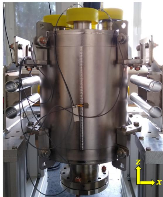
Figure 6: Mechanical resonances setup: four piezoelectric accelerometers mounted on the QPR's surface to measure vibrations in the  $x$ ,  $y$ , and  $z$  axes.
