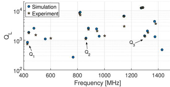
Figure 10: Loaded quality factor vs. Frequency of the QPR at room temperature. Comparison between simulation and experiment.
