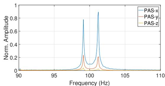
Figure 7: Normalized fast Fourier transform vs. Frequency. Three piezoelectric accelerometers (PAS) mounted on the top part of the QPR measured vibrations in the three dimensions when hitting it in the vicinity of the sensors.
