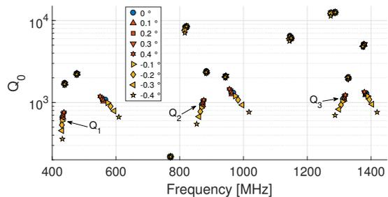
Figure 4: Quality factor vs. Frequency of the QPR at room temperature with a rotation of the rods around the  $y$ -axis at an angle  $\theta$  between  $-0.4^\circ$  and  $0.4^\circ$ .
