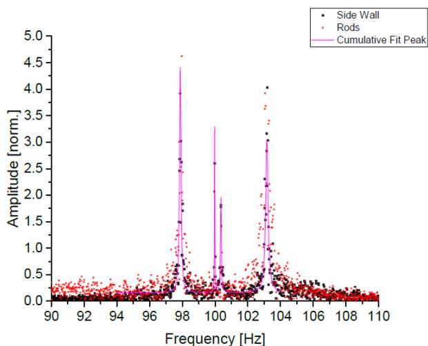
Figure 5: Normalized fast Fourier transform vs. Frequency. Mechanical spectrum of HZB's QPR measured with the geophone. Vibrational eigenmodes at and around 100 Hz are observed [14].
