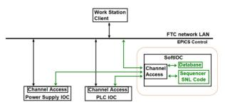
Figure 8: The IOC level program implement schematic.
