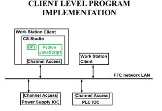
Figure 3: The client level program implement schematic.
