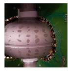
(b) Partially removed Tmap boards showing location of sensors on the cavity.
