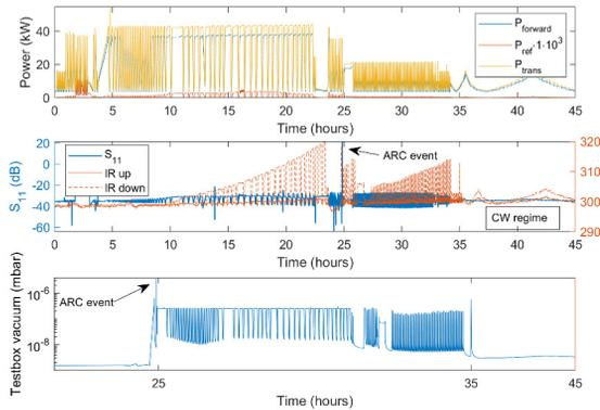
Figure 9: Part of the conditioning series of the 2<sup>nd</sup> coupler pair displaying peak power,  $S_{11}$  parameter, ceramic window temperature and testbox vacuum with time.
