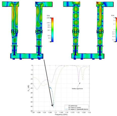
Figure 4: Top row displays the traveling wave field distribution for absolute electric (left) and magnetic field component (right) solved by 3DS CST FD solver normalized to  $0.5 W_{rms}$  input power. The lower plot depicts the  $S_{11}$  scattering parameter of the testbox with a pair of couplers mounted with normal CF gasket at the 5K port, RF sealed CF gasket (both measured by VNA) and the same using the Klystron as power source.
