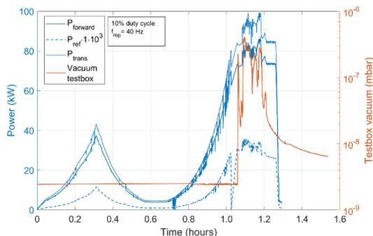
Figure 6: Intermediate result of first condition series with 1<sup>st</sup> pair reaching about 90 kW forward power at 10 % duty cycle with 40 Hz repetition rate displaying the three power signals and testbox vacuum with time.
