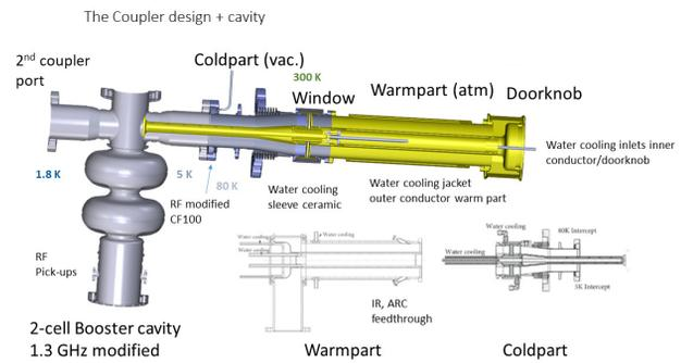
Figure 2: Schematic overview of the bERLinPro Booster injector coupler. The insert gives a better view on the water cooling channels and the diagnostic port observing the ceramic window.
