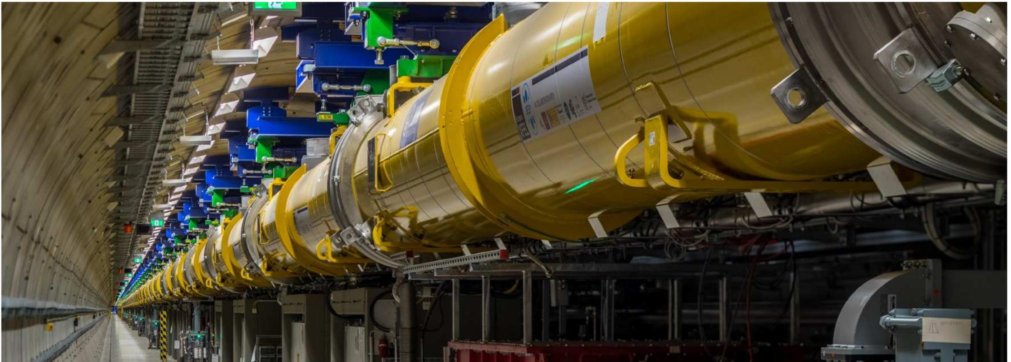
■ Worlds first long sc accelerator, 20 GeV, ~1000 m acc. length, 800 Nb cavities, 100 cryo-modules
