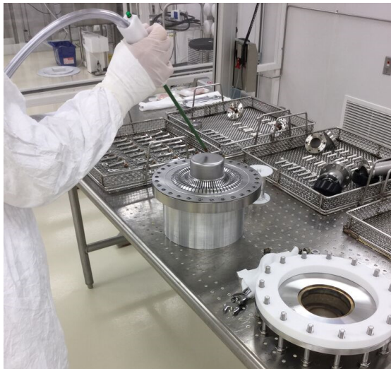
ISO 5 /Class -100 Surface particle counts of tuning plate
