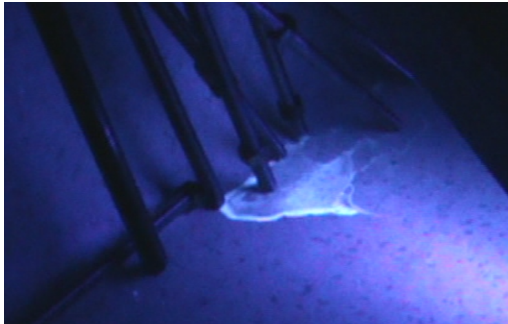
Detect detergents and water marks with UV light
