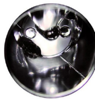
AFTER 12HRS OF EP 150µm Nb REMOVED
