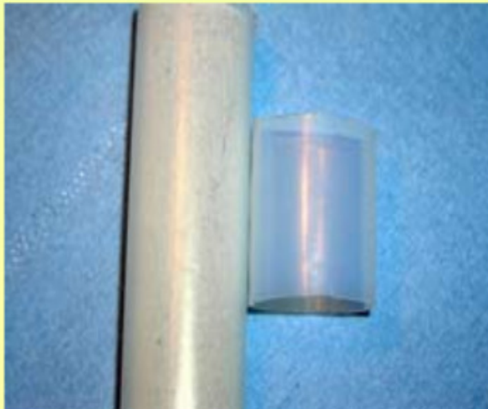
Tube before and after ethanol rinsing
