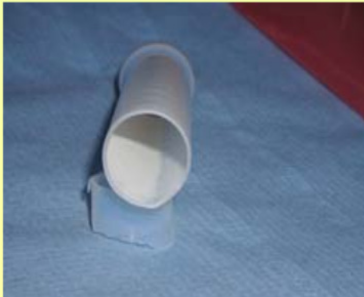
Tube with a thin sulphur layer
