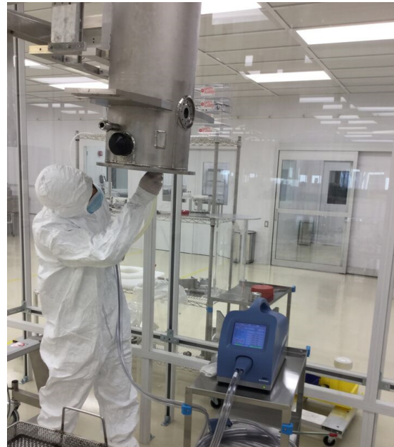
ISO 5 /Class -100 Surface particle counts of tuning plate
