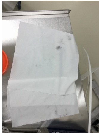
Grease from vacuum components
