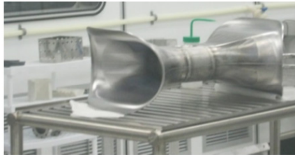
325 MHz Single-Spoke Fabricated at Niowave Inc.
