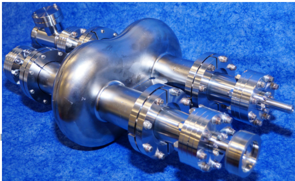
Twin axis cavity
