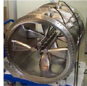
Superconducting RFQ Cavity
