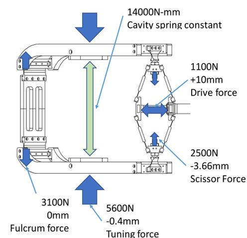
The forces and displacements on the SSR1 tuner components under maximum load. The mechanical advantage in force is 5:1 and the drive ratio is 25:1
