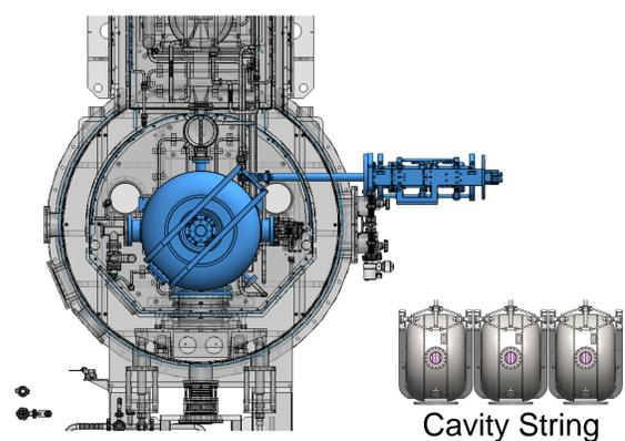
The SSR1 cavity and tuner installed in the SSR1 cryomodule.
