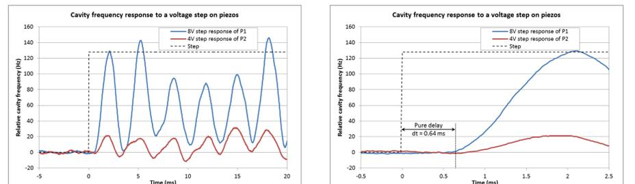
Pure delay has been measured using the same setup than for the transfer function. It is defined as the time between the beginning of a piezo action (voltage step on the piezo amplifier) and the beginning of the cavity frequency rising. It is imputed to the time travel of the acoustic wave from the piezo actuator to the cavity through the different mechanical parts of the tuner. The measurement of this parameter is also used to describe the numerical model of the tuner for simulation purpose.
