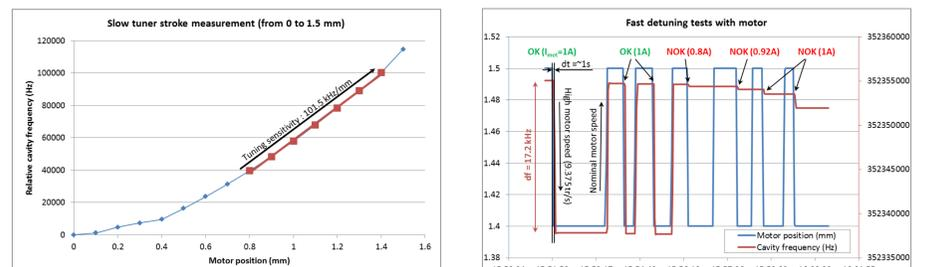
Slow tuner measurements consist of exploring the whole tuner range from 0 (when the tuner is not yet connected to the cavity) to 1.5 mm (when the tuner is fully connected to the cavity). From 0.2 to 0.4 mm the tuner is not fully connected to the cavity, this zone should not be used during operation because of strong non linearity, backlash issue and piezo response which would not be optimal.
