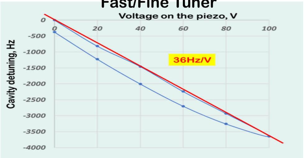
Per vendor specs warm piezo deliver stroke  $\sim 0.3 \mu\text{m/V}$  or 54Hz/V (with 180Hz/um).
