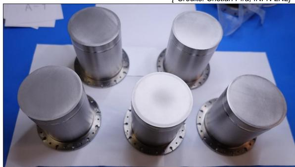
5 mechanically polished Nb substrates (before BCP)
