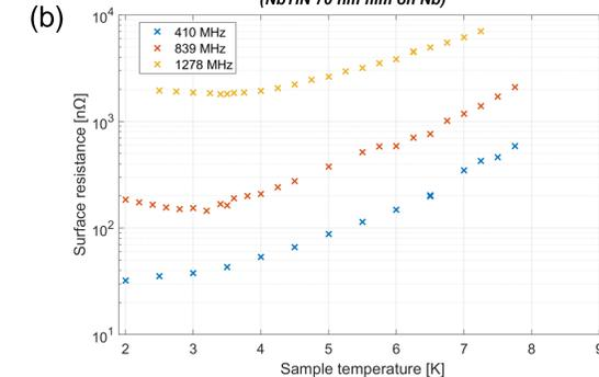
Surface resistance as a function of temp. for three modes (~9-10 mT) (SIS NbTiN sample, see also pres. by S. Keckert [3])
