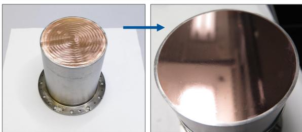
One of the Cu substrates after fabrication and after SUBU.
