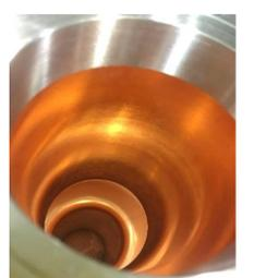
Chemical polished copper cavity substrate
