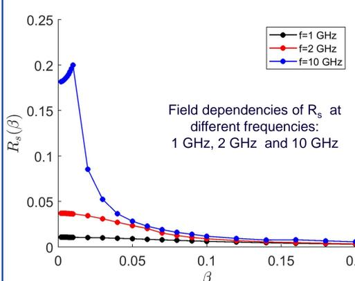
Field dependencies of  $R_s$  at different frequencies:  $1 \text{ GHz}$ ,  $2 \text{ GHz}$  and  $10 \text{ GHz}$
