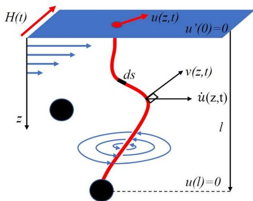
Dynamic equation for the local velocity normal to a flexible vortex line:
