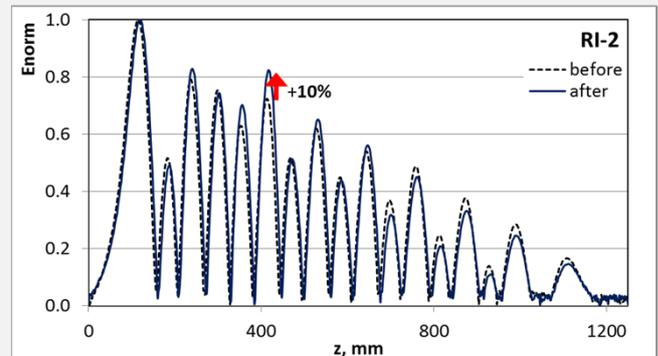
Figure 3: Normalized field distribution  $|E(r=0,z)|$  on cavity axis for second monopole mode TM011
