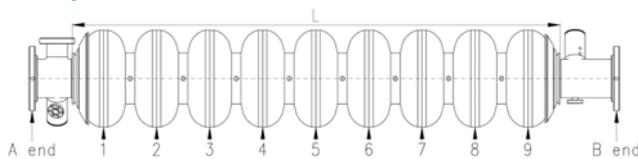
Figure 1: Length (L) of 9 cells LCLS-II cavity
