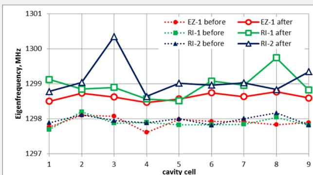
Figure 2: Cavity cells eigenfrequencies before and after rolling
