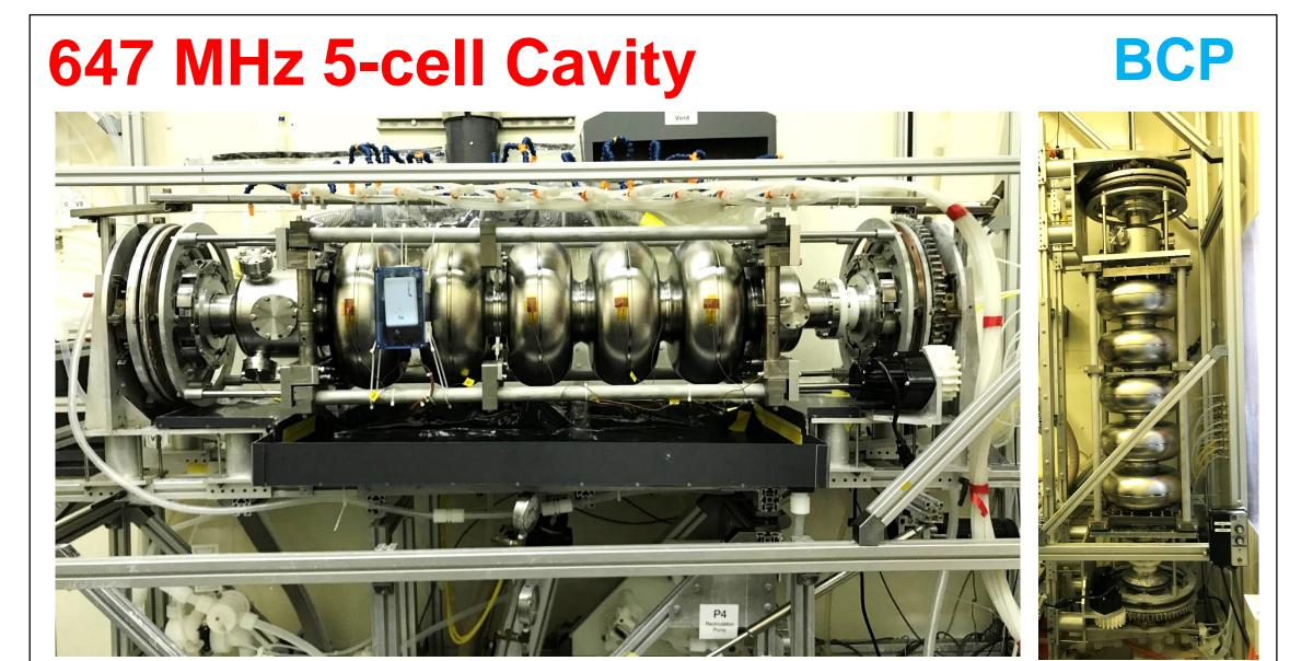
**Horizontal BCP and cavity rinsing**
