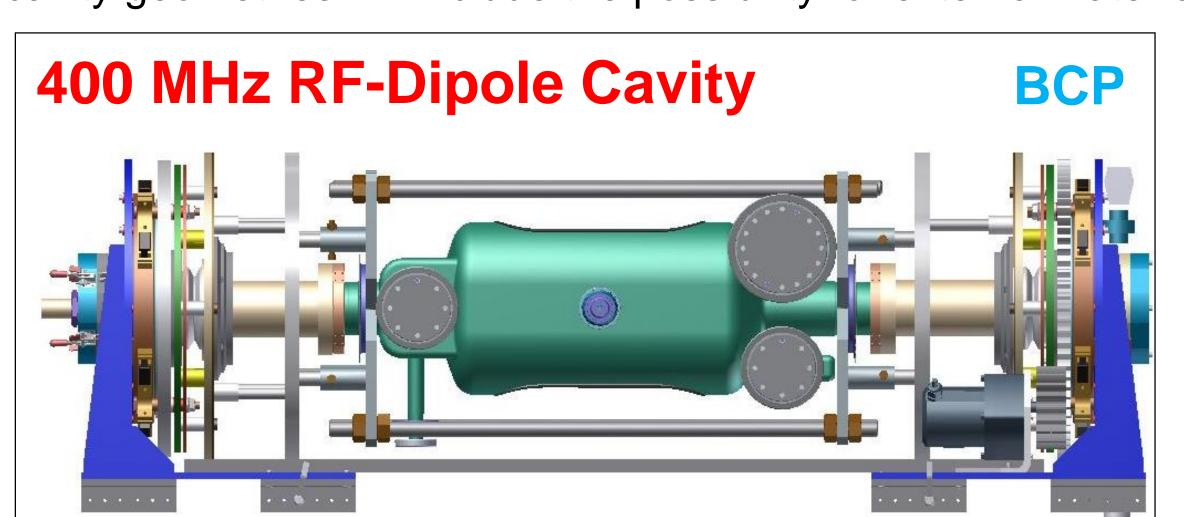
Proof-of-principle crab cavity for the High Luminosity Upgrade of the LHC at CERN, processed in collaboration with Fermilab/ODU.
