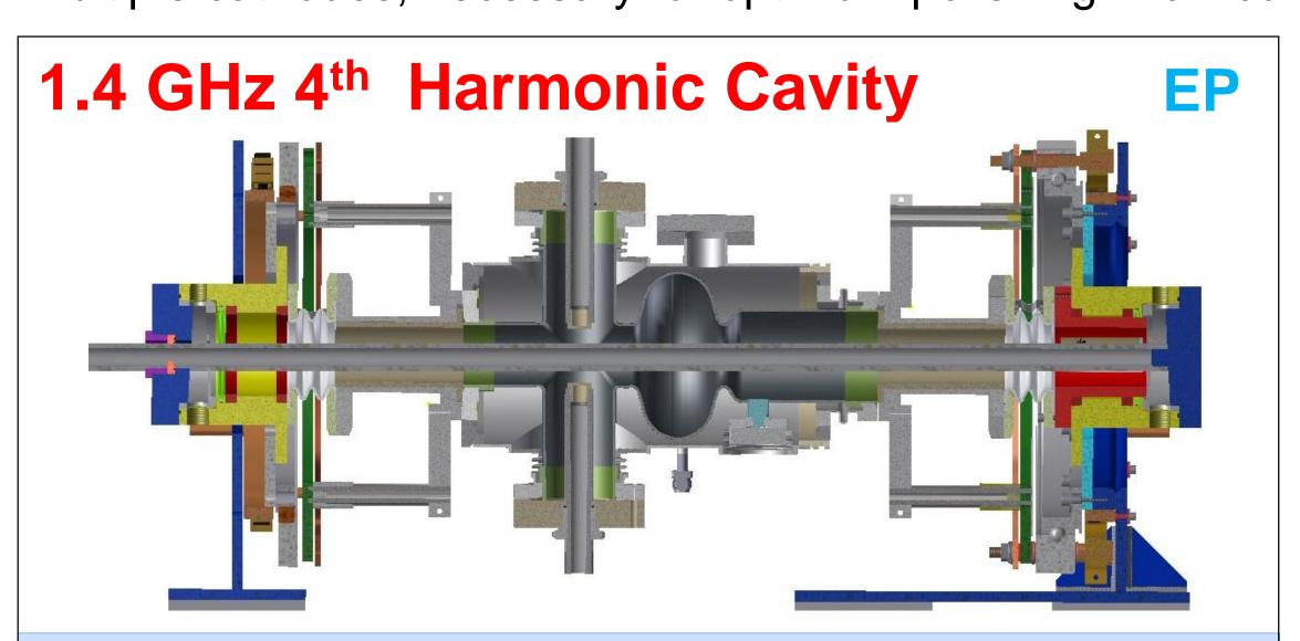
Key component of a single cavity bunch lengthening cryomodule for the Advanced Photon Source Upgrade at ANL.
