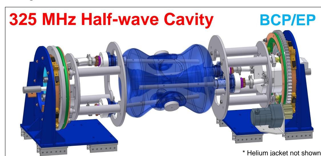
Compact half-wave cavity with highly optimized geometry, currently used for flux trapping and expulsion studies at ANL.
