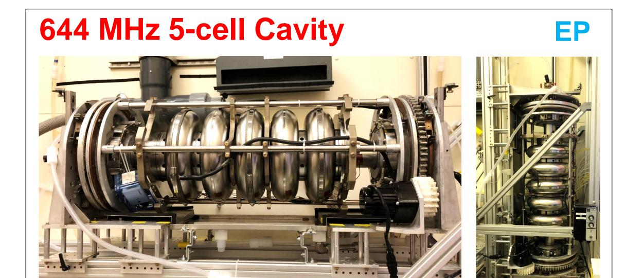
Horizontal EP and cavity rinsing
