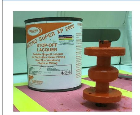
Left: Acid-resistant masking Bottom Left: EP mock setup
