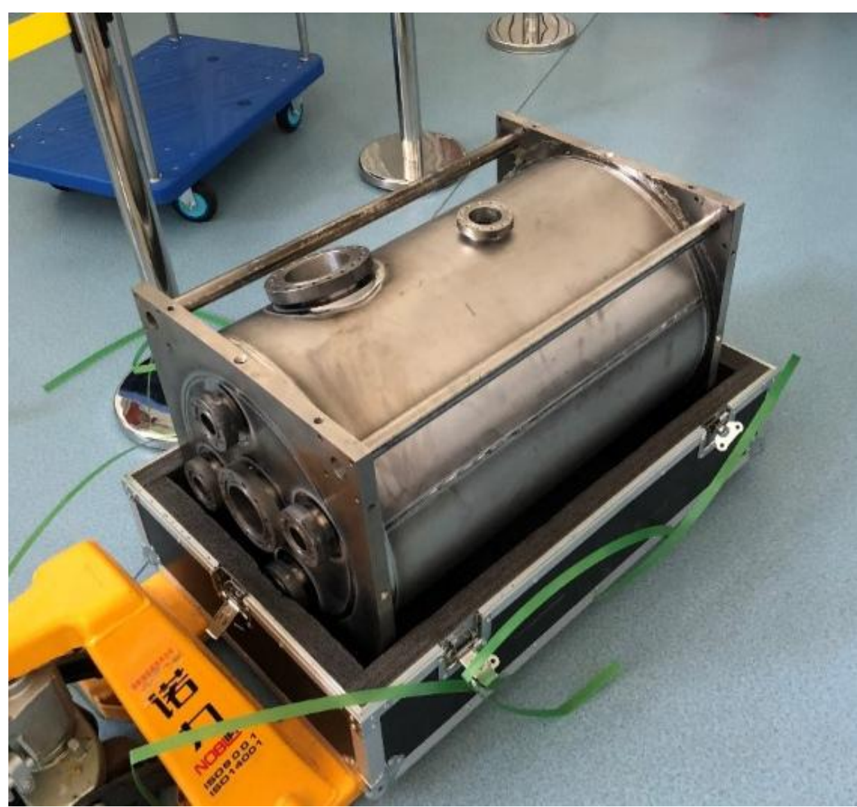
The fabricated LHe vessel
