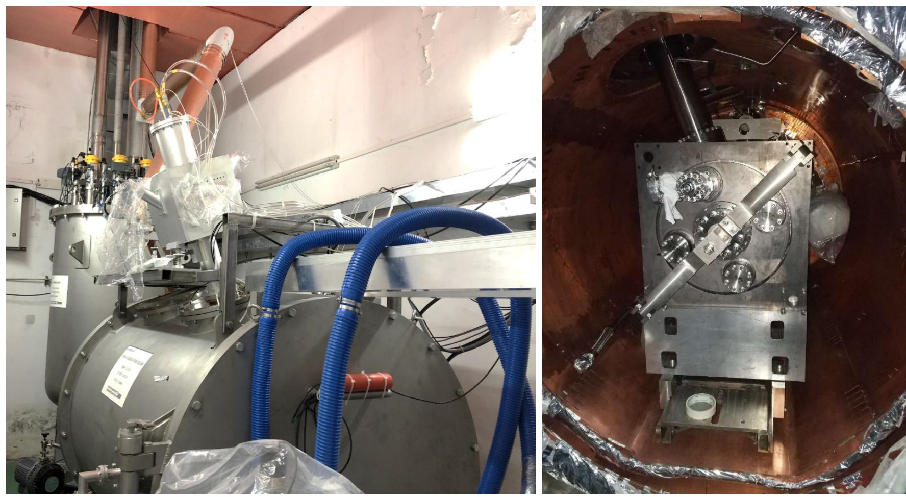
The dressed cavity installed in cryomodule
