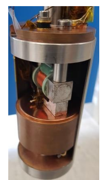
Figure 6 – The cage containing the sample and superconducting coil.
