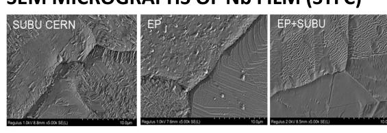
On STFC samples pitting is not visible because the Nb film is thicker than INFN and Siegen samples. (10  $\mu$ m instead of 3  $\mu$ m) Low deposition rate could help to mitigate substrate imperfections
