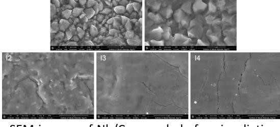
SEM images of Nb/Cu sample before irradiation (A) and after irradiation by Nd:YAG laser with intensities:  $I1 = 140 \text{ MW/cm}^2$ ;  $I2 = 170 \text{ MW/cm}^2$ ;  $13 = 253 \text{ MW/cm}^2$ ;  $14 = 320 \text{ MW/cm}^2$ .
