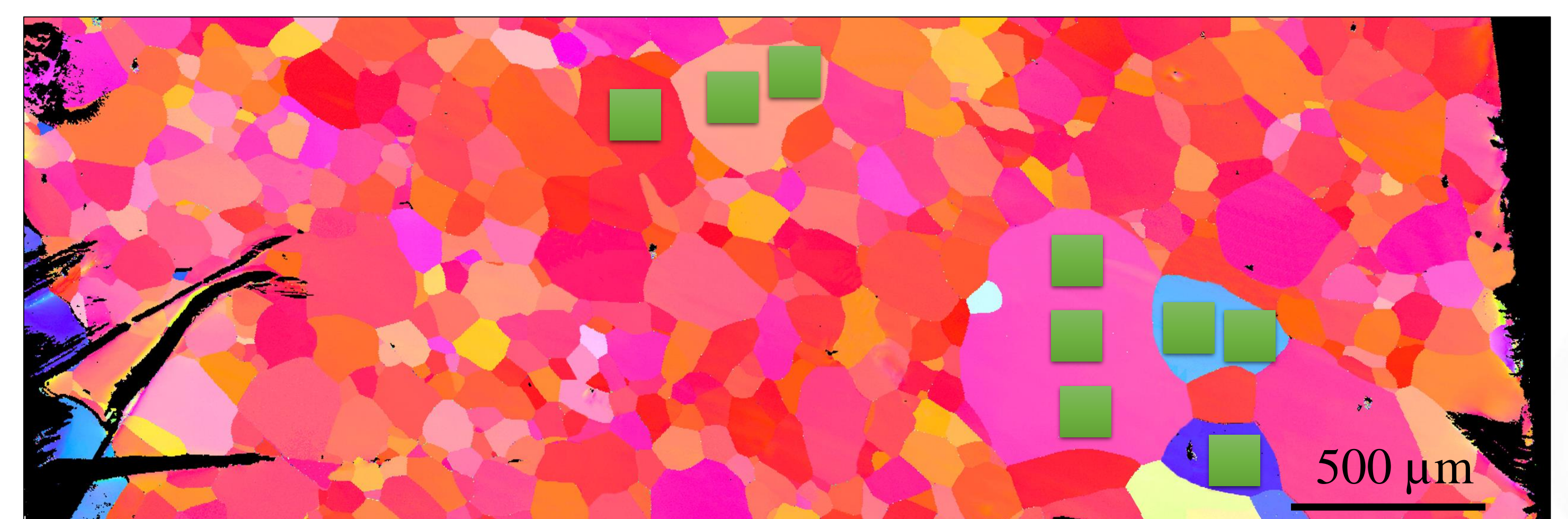
Top. EBSD map of a Sample with a [001] preferred surface orientation. Locations where SIMS analysis are performed are noted
