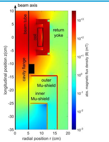
magnetic flux density inside shield material
