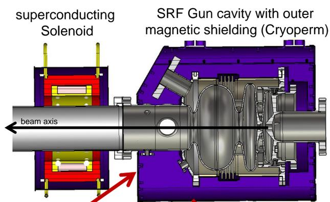
magnetic fringe field during magnet operation flows through the shielding of the cavity
