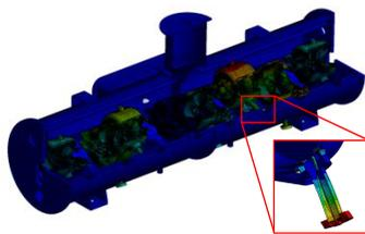
$$\begin{bmatrix} F_x \\ F_y \\ F_z \\ M_x \\ M_y \\ M_z \end{bmatrix} = \begin{bmatrix} \dots \\ \dots \\ \dots \\ \dots \\ \dots \\ \dots \end{bmatrix} K \begin{bmatrix} U_x \\ U_y \\ U_z \\ \theta_x \\ \theta_y \\ \theta_z \end{bmatrix}$$
