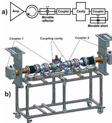
Figure 11: a) RF scheme of 650 MHz coupler test facility; b) 3-d model of test bench b).
