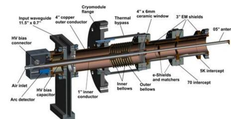
Figure 6: Cut view of 650 MHz coupler with electromagnetic shields.
