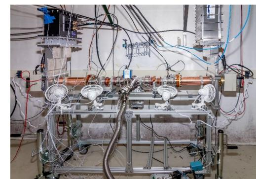
Figure 12: 650 MHz coupler test bench.
