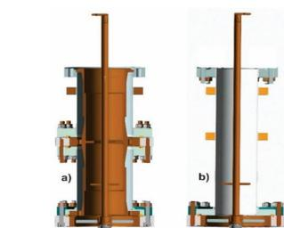
Figure 7: Cut views of vacuum parts of 650 MHz coupler with electromagnetic shields (a) and of conventional coupler with copper coating (b).
