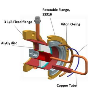
Figure 2: Window unit, first design.
