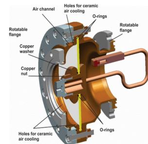
Figure 3: Window unit with replaceable ceramic, second design.
