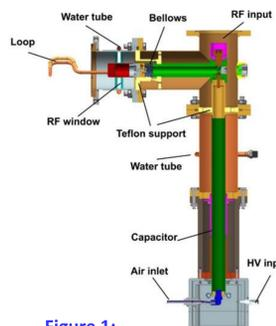
Figure 1: Configuration of RFQ coupler
