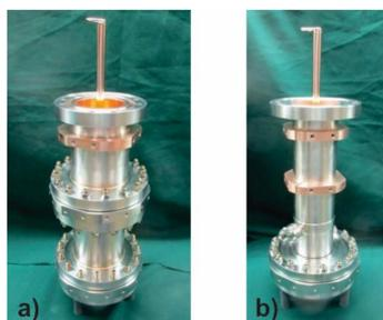
Figure 10: Appearance of outer conductors with coppers shields, a) and outer conductor with copper coating, b).
