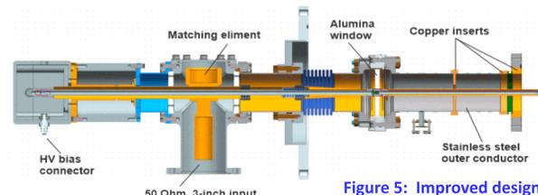
Figure 5: Improved design of 325 MHz coupler.
