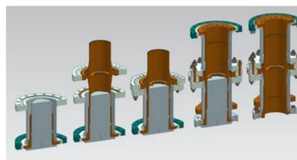
Figure 8: Assembly sequence of outer conductor with copper shields using Teflon jig.
