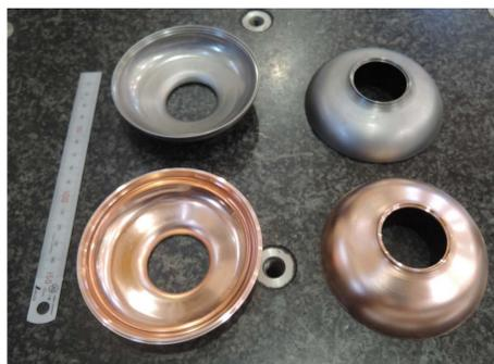
Trimming of Cu and Nb cups at KEK. Trimming fixture were designed and fabricated at Jlab
