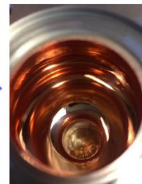
Two Cu cavities: Mechanical polishing (CBP: Centrifugal Barrel Polishing) at JLab
