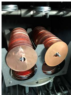
Annealing of Cu (C1020) disks in vacuum furnace at KEK ( 520 C x 2 hours )
