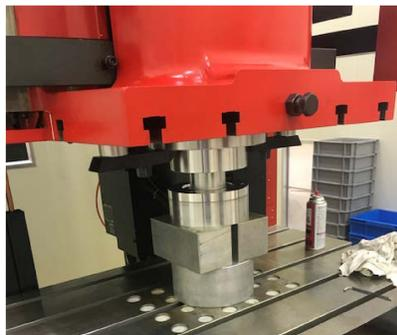
Nb plates were produced by Tokyo Denkai. Press-forming of cups at KEK. Press dies were designed and fabricated at Jlab
