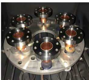
Brazing of stainless-steel flanges and Cu beam-pipes. Brazing: Ag 72.5% , Cu 27.5%, others < 0.15%
