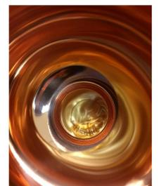
Seven 3.0-GHz Cu cavities were fabricated at KEK and two of them were sent to Jlab for surface preparation. Plan: Nb-film creation on the inner-surface by KEK or Jlab, and performance test (vertical test) at Jlab.
