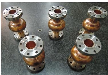
Seven Cu cavities were fabricated by a NEC 6-kW EBW machine at KEK. EBW parameters: Iris (V = 80 kV, Speed = 10 mm/sec, I1 = 15 mA, I2 = 29-31 mA) Equator outside (V = 80 kV, Speed = 10 mm/sec, I1 = 15 mA, I2 = 23-25 mA) Equator inside (V = 80 kV, Speed = 10mm/sec, I = 17-18 mA)
