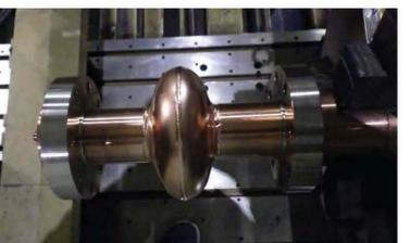
Two 3.0-GHz Cu cavities were fabricated at a company.
