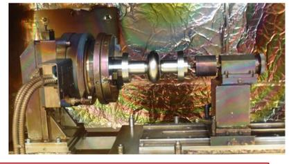
Mitsubishi Electric Low-Voltage-type EBW machine: EBW parameters. Nb-Ti flange + Nb beam-pipe: 60 kV, 12 mA
