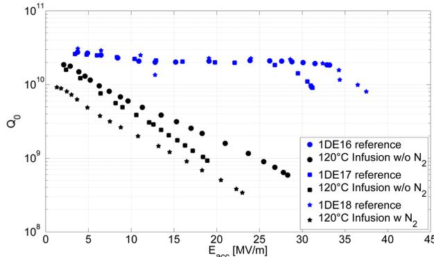
Figure 1: Quality factor vs. accelerating field of the first three single cell cavities used for infusion R&D. Reference measurements (blue) and measurements after treatment (red) are shown. The same deterioration for all cavities are observed.
