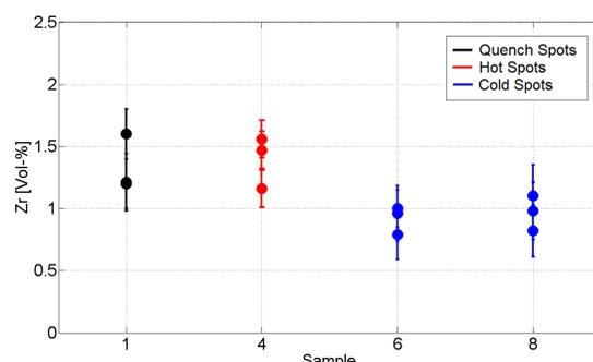
Figure 6: Zirconium concentration for some samples according to PIXE. A slightly higher concentration in the hot spot and quench spot samples compared to the cold spots samples was found.
