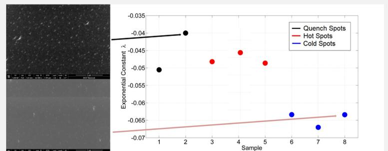
Figure 4: SEM Images of sample 2 (top – quench - black) and 8 (bottom - cold post - blue). The right plots shows the exponential decay constant  $\lambda$  of the size distribution of the niobium carbides.
