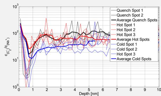
Figure 3: Normalized C<sub>2</sub><sup>-</sup> - signal of each sample in the first 10nm obtained with a TOF-SIMS. Quench spots and hot spots showed a higher carbon content in this first layer.
