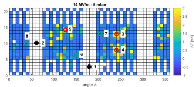
Figure 2: Temperature map of 1DE16 – white squares are the position of the H-Map cards. A rather homogenous heating with only three dominant heating spots is observed.
