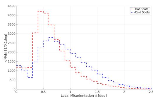
Figure 5: Local misorientation data for hot spots (red) and cold spots (blue). Average over 2 measurements per sample, covering a 200x150 grid with a 10  $\mu$ m step size. An excess of low angle grain boundaries for hot spots compared to cold spots was found.
