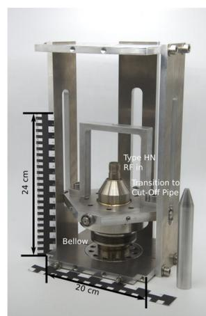
New input coupler before final cleaning and assembly. The coupler is mounted on top of the cavity, allowing variation of the coupling strength.
