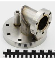
New output coupler with Type N RF out and cavity vacuum pumping flange, upgrading from the previous CF16 diameter to CF40 allowing better vacuum performance.
