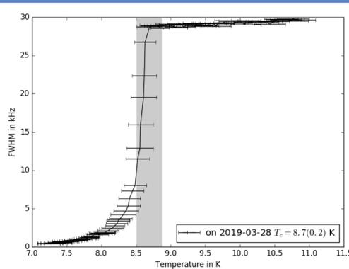
FWHM of the single cell cavity during cooldown. Below the critical temperature  $T_c = 9.25$  K of Nb, a steep change of the slope occurs as the FWHM is drastically reduced due to the transition to the superconducting phase. This can be used as an first indication of a successful  $\delta$ -NbN growth ( $T_c = 16.2$  K).
