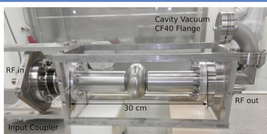
Clean room assembly of a single cell 3 GHz cavity in the new vt insert. Left of the cavity is the variable input coupler (top in vt), right of the cavity the new output coupler with CF40 cavity vacuum flange.
