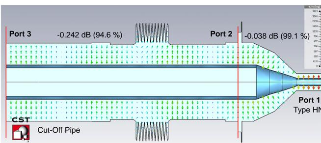
Input coupler simulation of S-Parameters optimizing the geometry of the transition from Type HN RF input vacuum feedthrough ( $r_i=2.4$  mm,  $r_o=5.6$  mm) to cavity cut-off pipe ( $r_i=11$  mm,  $r_o=25$  mm).
