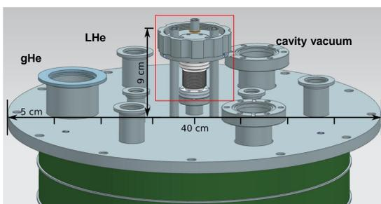
New head cover with 40 mm cavity vacuum pumping ports, multiple ports for instrumentation, LHe support and gHe outlet. In the center is the custom nut for controlling  $Q_{ex}$  of the input coupler.
