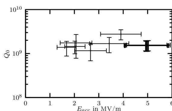
Preliminary  $Q_0$  vs.  $E$  measurement at  $T=2$  K of a single cell cavity with the new vertical bath cryostat insert using a decay time method. During the measurement, the rf forward power did not exceed 1 W, the dissipated power at 5 MV/m is 400 mW.
