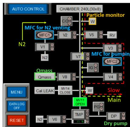
Figure 7: Block diagram of the slow pumping system.
