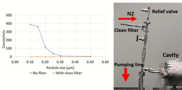
Figure 5: Particle measurement at the nitrogen purge unit.
