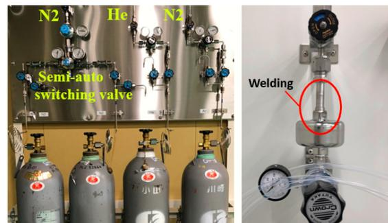
Figure 4: Gas source handling panel and gas outlet.
