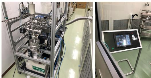
Figure 6: Slow pumping system and operation panel.
