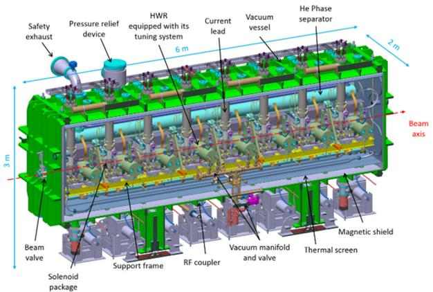
Figure 1: Schematic view of LIPAc cryomodule.
