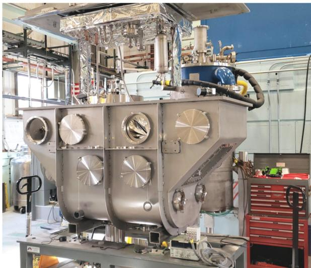
Figure 1: Top-loading 2-meter long bunch lengthening cryomodule.
