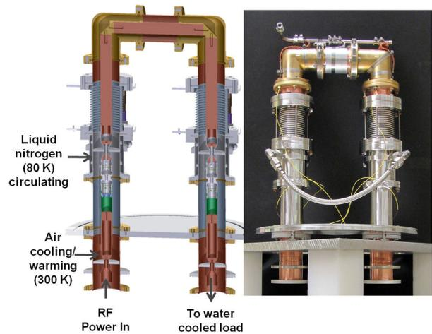
Figure 5: Test stand configuration for a pair of fundamental RF power couplers.
