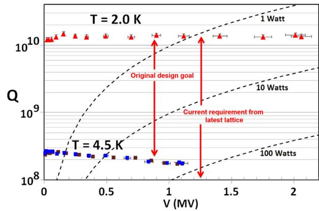
Figure 3: Cavity performance curves at 2 K and 4.5 K.
