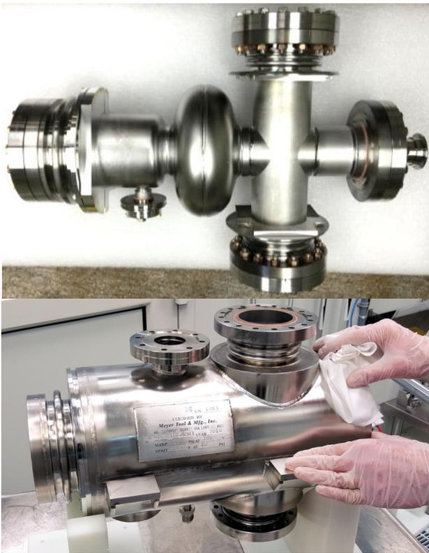
Figure 2: Niobium cavity subassembly (top) and production-ready higher-harmonic cavity (bottom).
