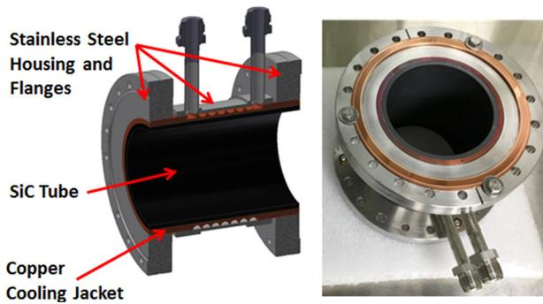
Figure 4: Higher order mode damper assembly.
