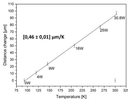
Figure 9: Movement of the insert with increasing thermal load.
