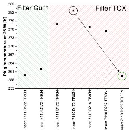
Figure 10: Overview of the tested components with different spring configurations for a heat load of 25 W with respect to the plug temperature.
