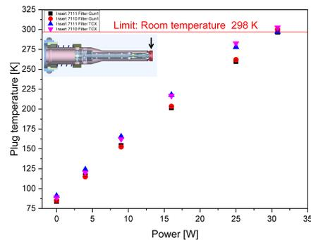
Figure 7: Different plug temperatures at different powers for two inserts and two RF-filters.
