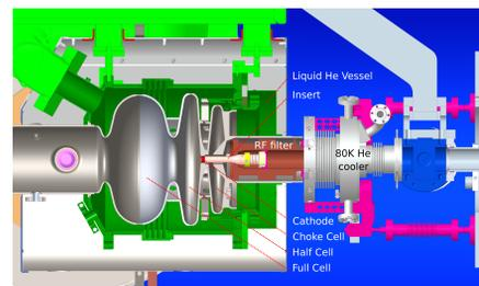
Figure 1: Cross section of the SRF photoinjector showing the cavity geometry together with the cathode section [5].
