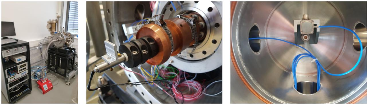
Figure 5: Overview of the TCX-setup: (left) Vacuum chamber, (center) Insert inside the RF-filter with heater and sensors and position marker for distance measurement, (right) distance sensor.
