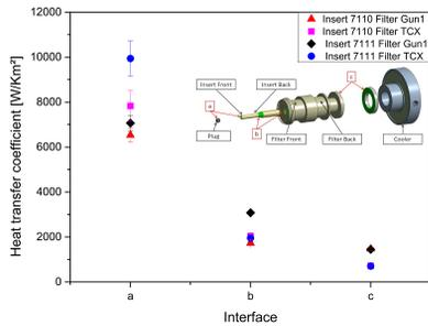
Figure 8: Heat transfer coefficients calculated for each thermal contact.
