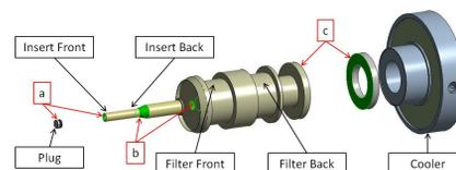
Figure 2: Three interfaces: a - plug/insert, b - insert/RF-filter, c - RF-filter/cooler.
