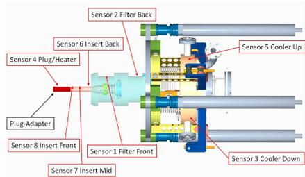
Figure 4: 3D-drawing of the thermal contact experiment.
