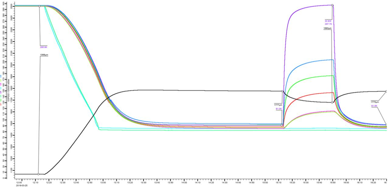
Figure 6: An example plot of the thermal contact measurement procedure. First the experiment is cooled down with liquid nitrogen until the equilibrium is reached. The movement of the cathode insert can be followed via the signal from the distance sensor (black). After the equilibrium is reached, the power of the heater was raised until room temperature is reached at the plug, which also causes movement in the opposite direction.
