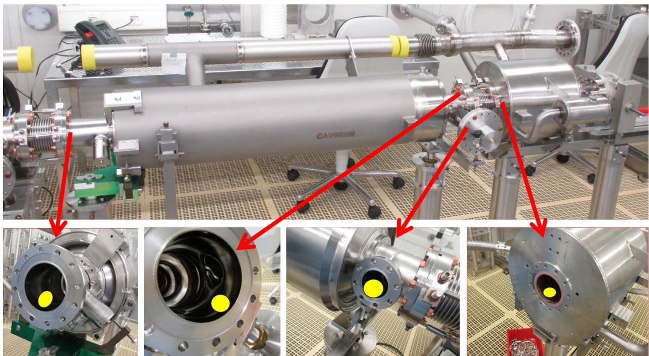
Figure 2: Cavity string in the DESY SRF clean room. The yellow spots represent the positions where the samples have been taken.
