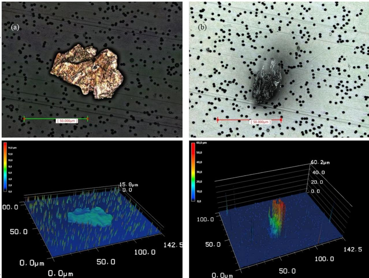
Figure 5: LSM analysis of (a) a Copper and (b) an organic particulate.
