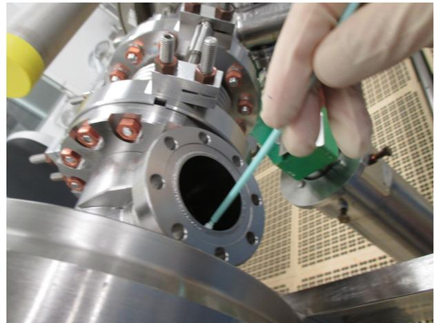
Figure 3: Swabbing contaminations from cavity main coupler port.
