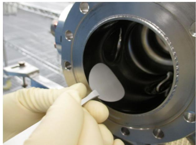
Figure 4: Insertion of a filter disc with plastic tweezers.
