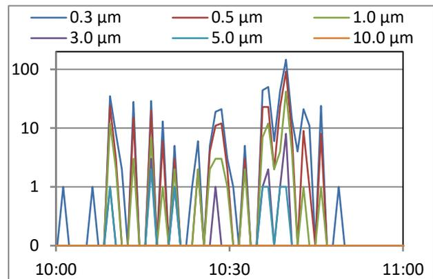
Figure 1: Typical particle count (measured in 1 minute interval) during the disassembly of a bellow between two cavities.
