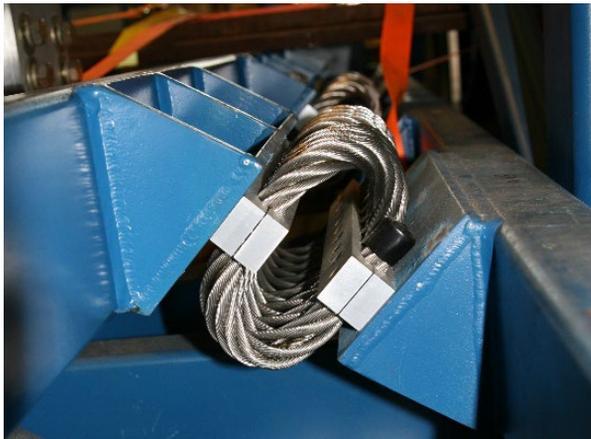
Figure 4: Helical isolator springs used on shipping frame.
