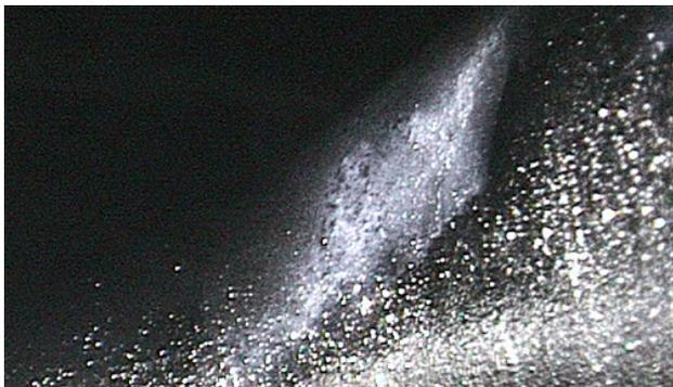
Figure 4: An example of acid vapour oxidation seen after a bulk etch process.
