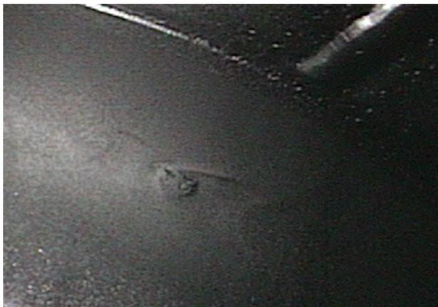
Figure 3: Borecope image of an etching feature that formed during the bulk etching process due to the close proximity of the end of the acid quill to the short plate.
