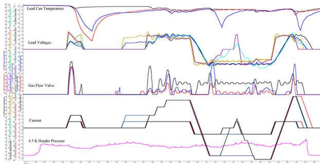
Figure 4: The CB10 solenoid's commissioning details.
